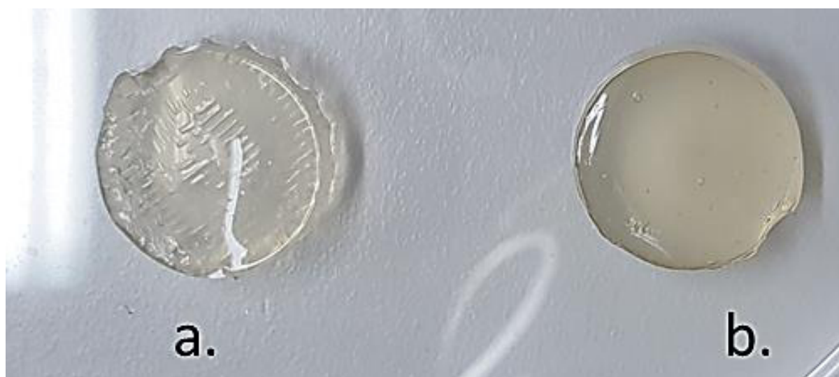
Figure 4. 3 Images of typical 3D printed SA-GL tablet-shaped matrices produced using a 3D Bioplotter in the least and most favourable concentrations: a. Least favourable printing ink (5%SA-8%GL) and b. Most accurate printing ink (8%SA-10%GL)
