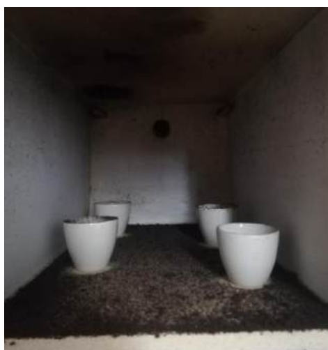
Figure 5.6: The samples prepared using [M T ]:[Cit] of 1:0.833 and 1:0.667 heated to 380 °C and calcined for 5 hours in air.
