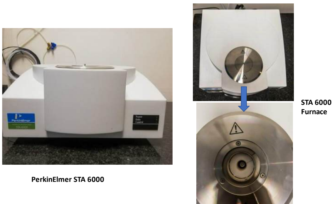
Figure 3.2: PerkinElmer STA 6000 used for thermal analysis with the bottom right picture showing the compact furnace.
