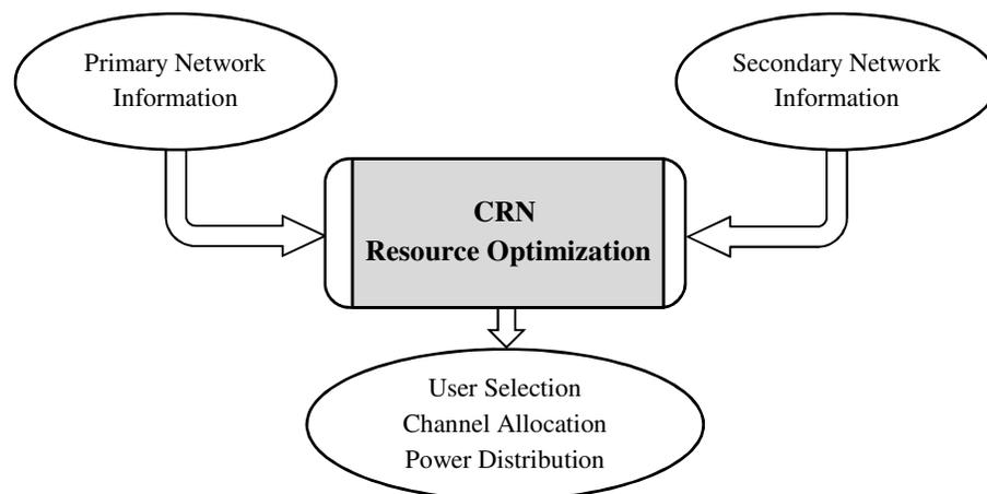
**Figure 1-2: Resource allocation and optimization process in CRNs.**
