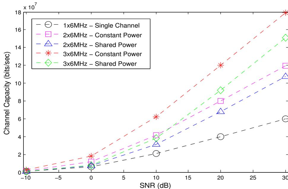
**Figure 2-4: Illustration of the impact of power allocation on ChA techniques.**
