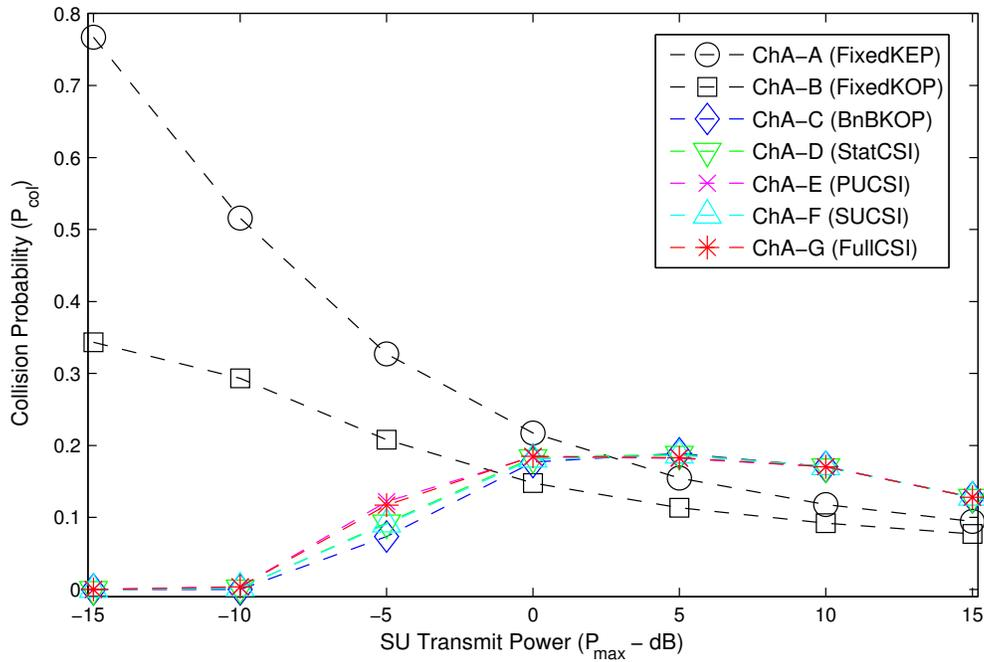
Figure 5-7: Collision probability versus SU total transmit power.
