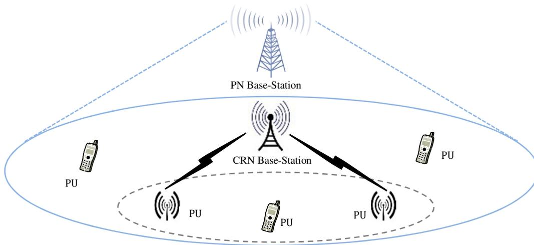
**Figure 6-1: Network model for infrastructure based multiuser multichannel CRN.**
