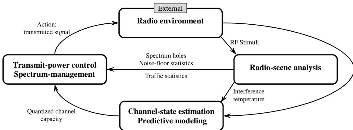
Figure 1-1: Basic cognitive radio functions and operational cycle [13].
