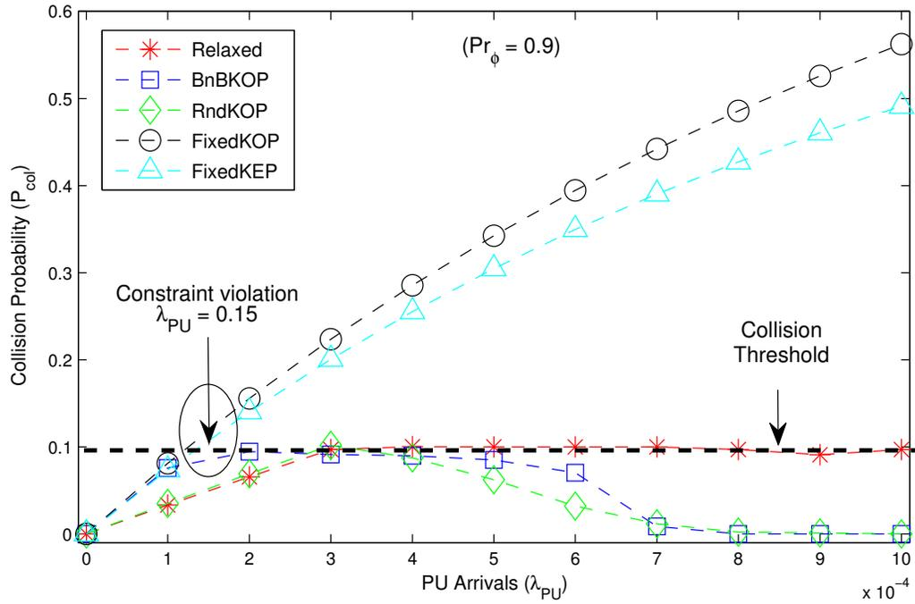
Figure 3-8: SU collision probability for increasing PU arrival rates at  $\mathcal{P}_{\phi} = 0.9$ .
