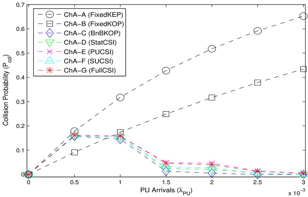
Figure 5-4: Collision probability for increasing PU arrival rates.
