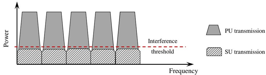
**Figure 2-2: Example of underlay spectrum access in CRNs.**
