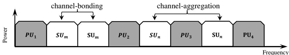
Figure 1-3: Illustration of channel-bonding and channel-aggregation.
