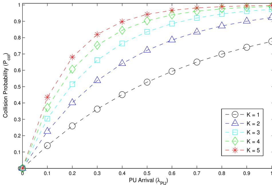
**Figure 3-2: Collision probability between PU and SU services for increasing PU arrival rates.**
