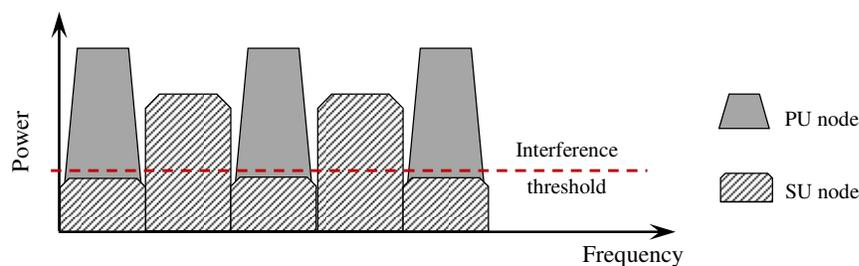
Figure 2-3: Example of hybrid spectrum access in CRNs.
