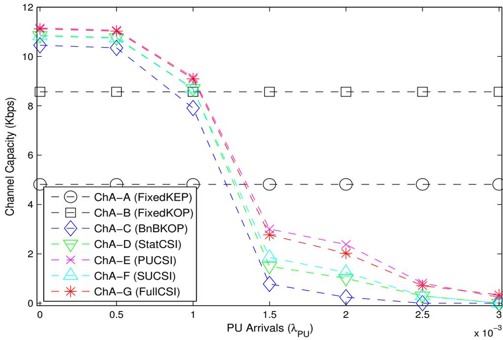
Figure 5-2: Channel capacity for increasing PU arrival rates.
