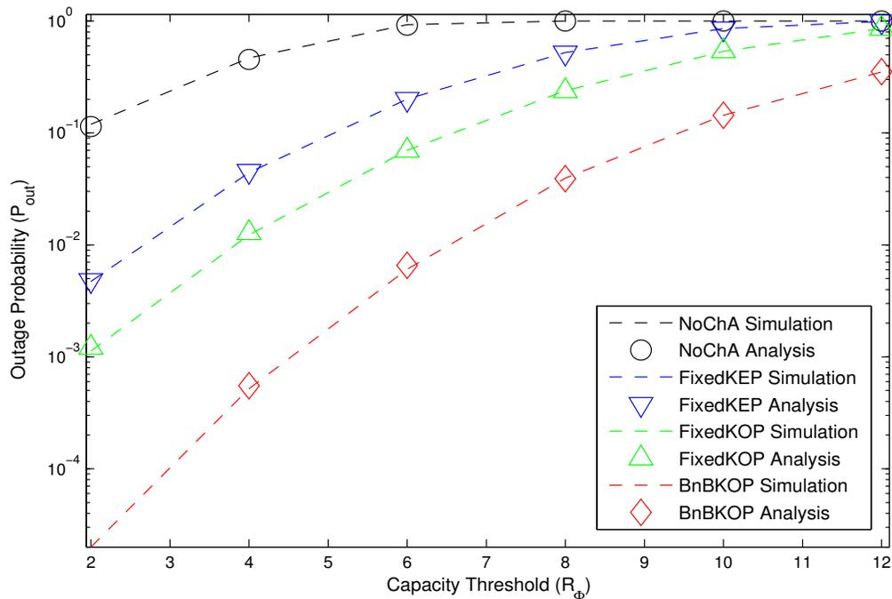
Figure 4-7: Outage probability against capacity threshold.
