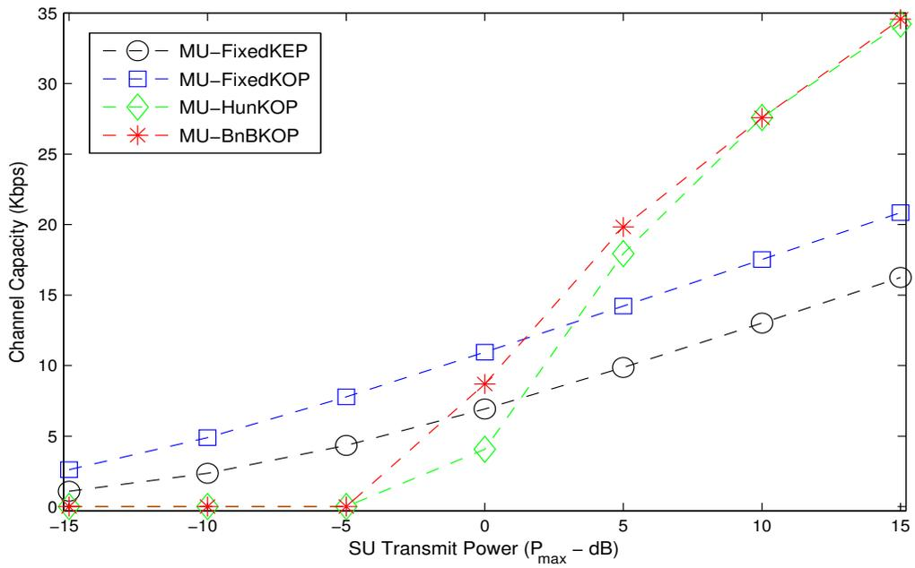
Figure 6-5: SU average capacity vs total transmit power.
