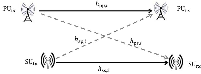
**Figure 5-1: Network model for hybrid overlay and underlay SU transmissions.**
