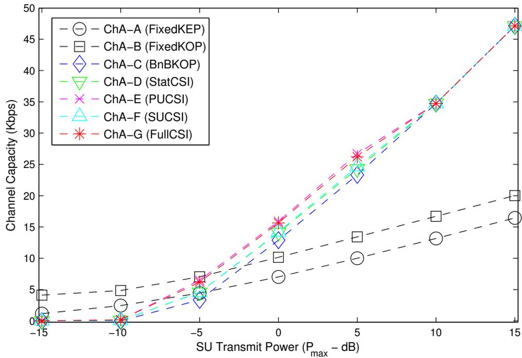
Figure 5-5: SU channel capacity versus SU total transmit power.
