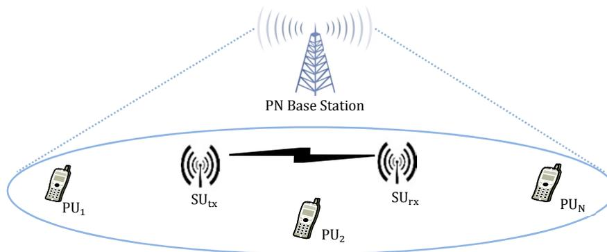
Figure 3-1: Network model for coexistence of a PN and CRN.
