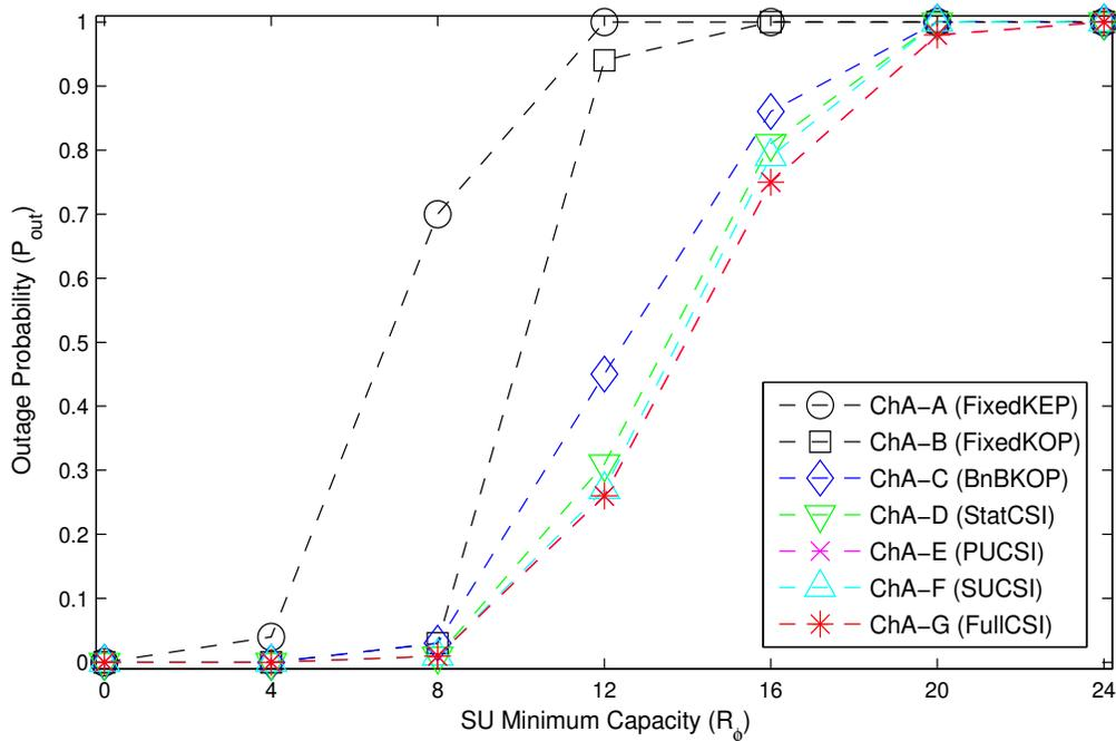
Figure 5-8: Outage probability versus SU QoS requirement on capacity.
