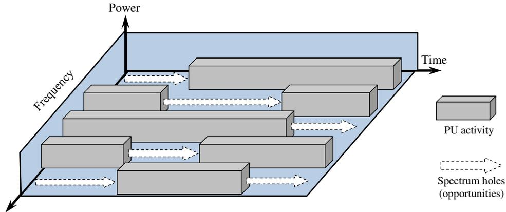
Figure 2-1: The concept of spectrum holes in CRNs.
