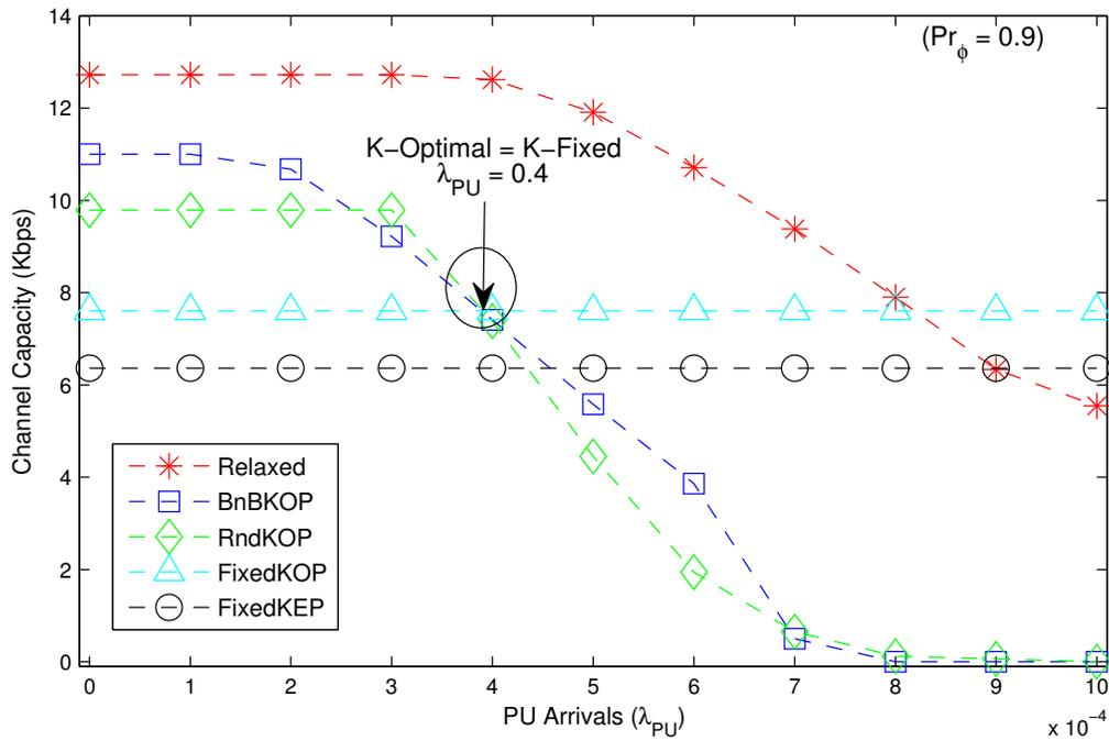
Figure 3-4: SU average capacity for increasing PU arrival rates at  $\mathcal{P}_\phi = 0.9$ .
