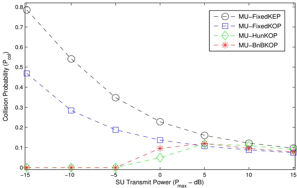
Figure 6-7: SU collision probability vs total transmit power.
