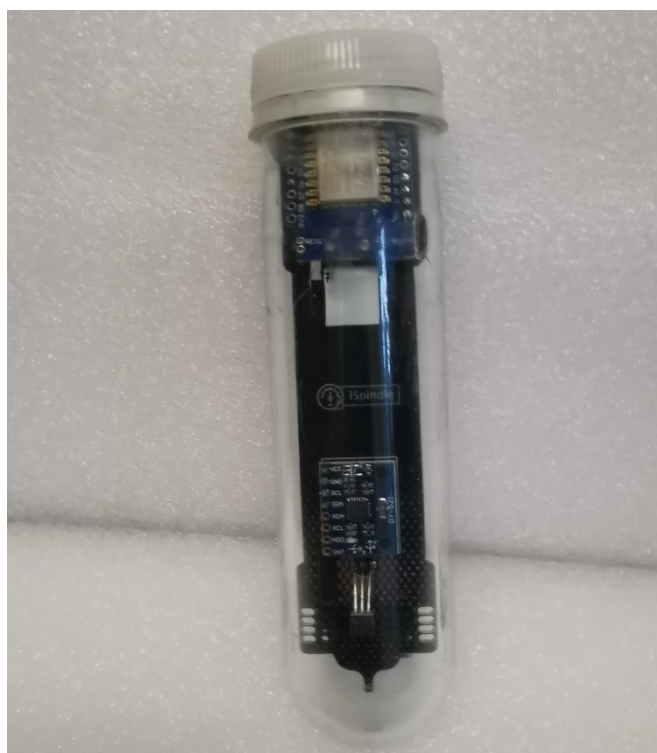
Figure 4.2: iSpindle device for measurement of density
