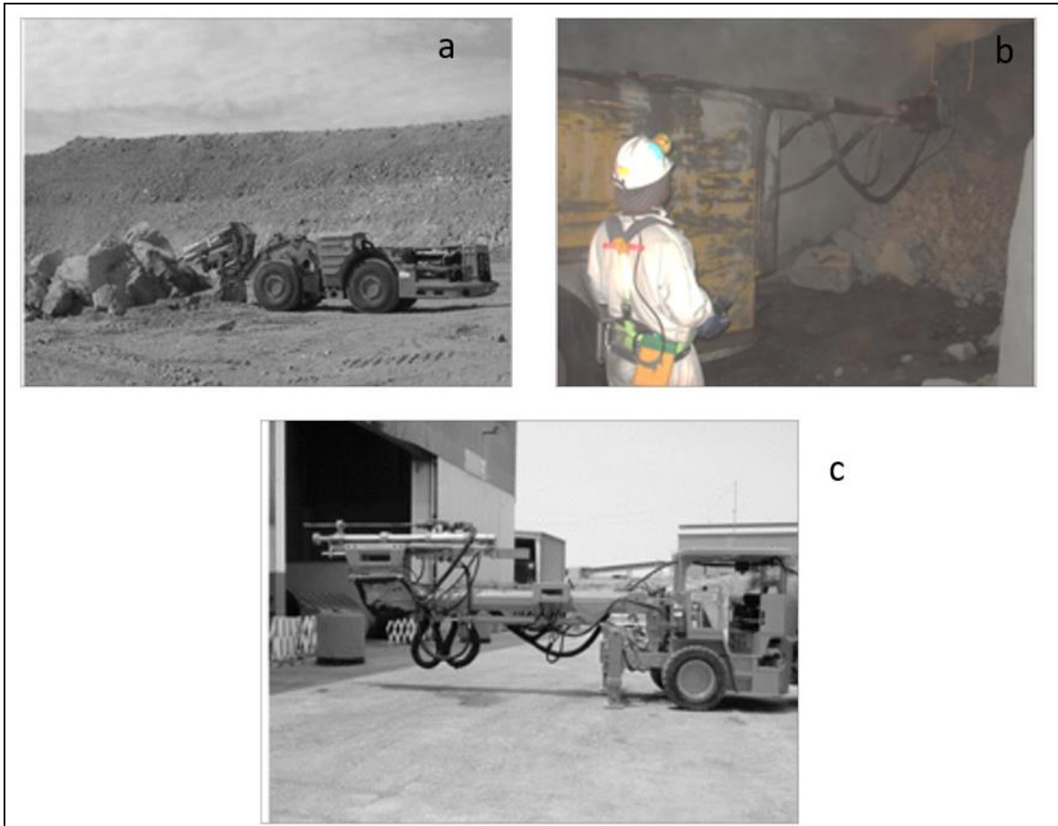
Figure 1.5: Mobile rock breaker hammering boulders (a), water cannon treating a hang-up underground (b), and a new medium reach rig at the workshop (c) (PalaboraMiningCompany, 2015)
