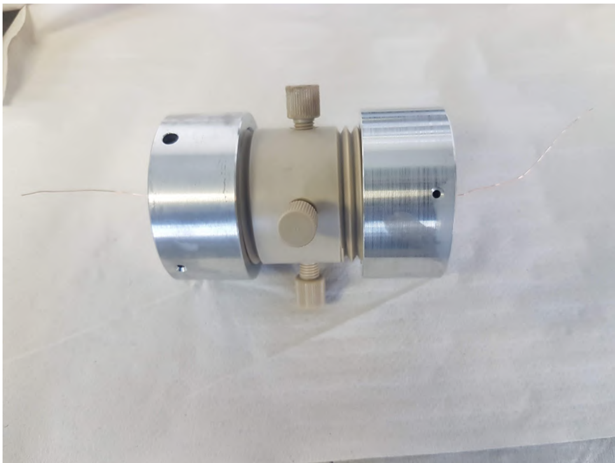
Figure 3.15: An image of the T-type Swagelok cell used in this work.
