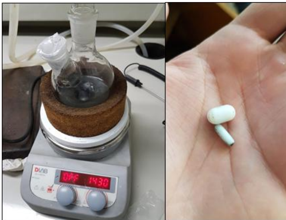
Figure 3.1: Set up for etching of MXene showing MAX phase in solution with LiF and HCl on a magnetic stirrer (left), and stir bar used for the magnetic stirring (right).
