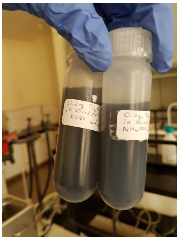
Figure 3.4: MXene in KOH and \text{NH}_4\text{OH} solution after shaking treatment for 90 hours.
