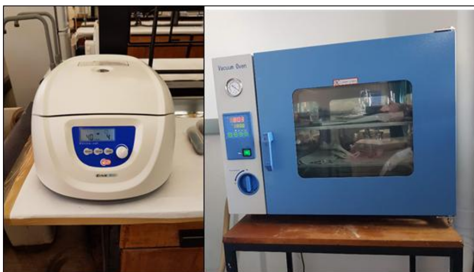
Figure 3.2: Centrifuge used for washing the MXene post-etching (left), and the vacuum oven used for drying the MXene after washing (right).
