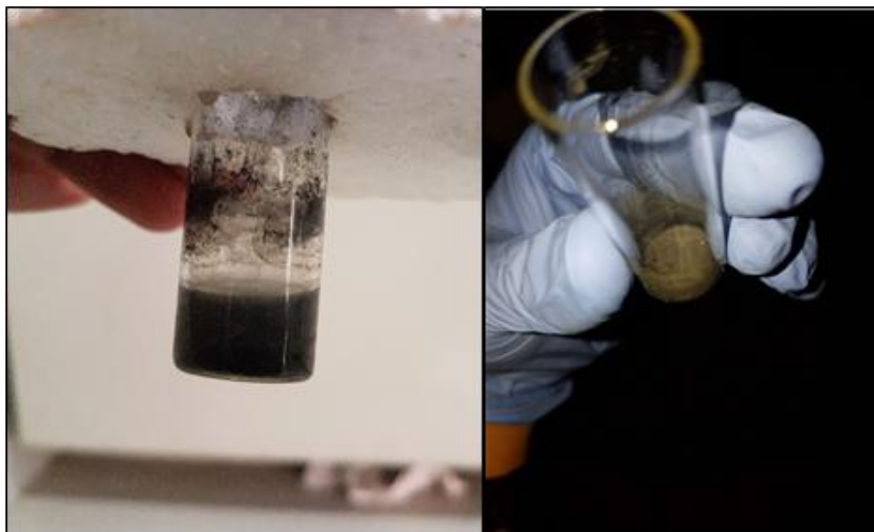
Figure 3.3: OLC doped MXene after sonication in DMF (left), and after drying in a vacuum oven (right).
