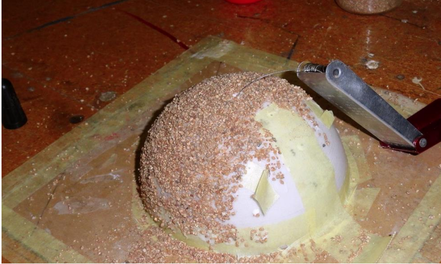
Figure 36: Glue Sand Particles to 3D Models
