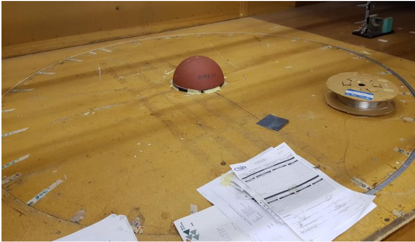
Figure 28: Dome model placed on turn table for testing
