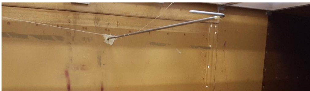
Figure 27: Pitot Static Tube (placed 750mm above the turn table)
