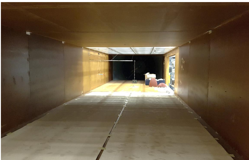
Figure 29: Corrugated Cardboard within 16m Fetch for Boundary Layer Simulation
