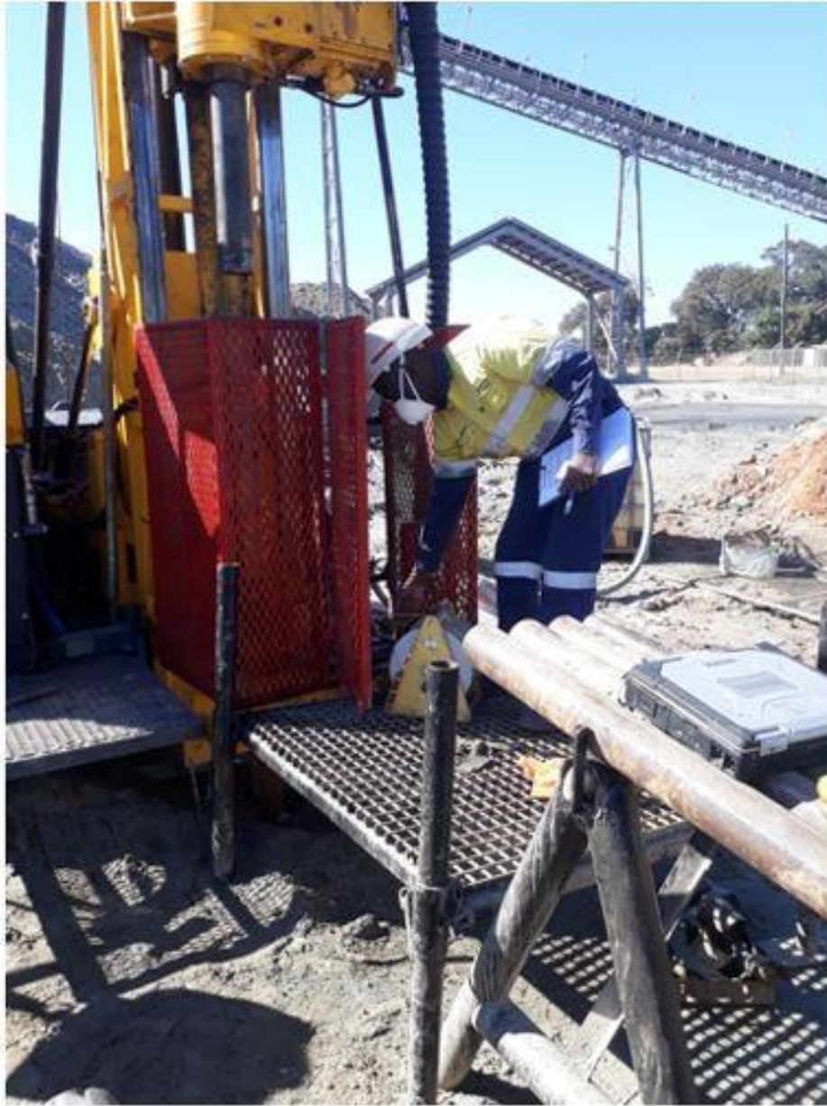
Figure 3.4 Falling Head test on an open diamond drill hole at Lumwana Mine.
