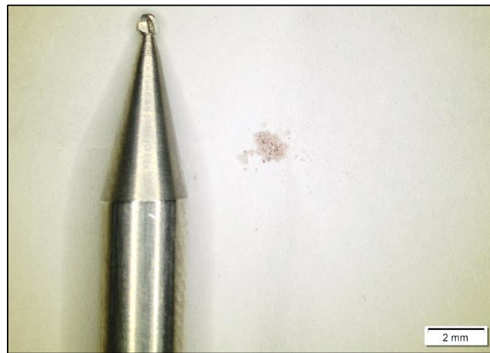
Figure 3.6: Tungsten Dremel drill bit with the \sim 400\ \mu\text{g} sampled bone fragment powder. This is sufficient for Ca isotope analysis.
