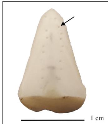
Figure 3.8: An adult female Crocodylus niloticus tooth, sampled using the micro-drill to perform calcium ion-exchange chromatography at ENS, Lyon. The black arrow (sample spot 8b) indicates a sample spot ~500 \mu\text{m} in diameter.
