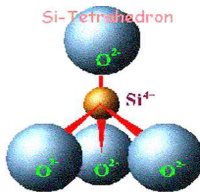
Figure 2.5: The structure of tetrahedral silicate (Kozák et al., 2010)
