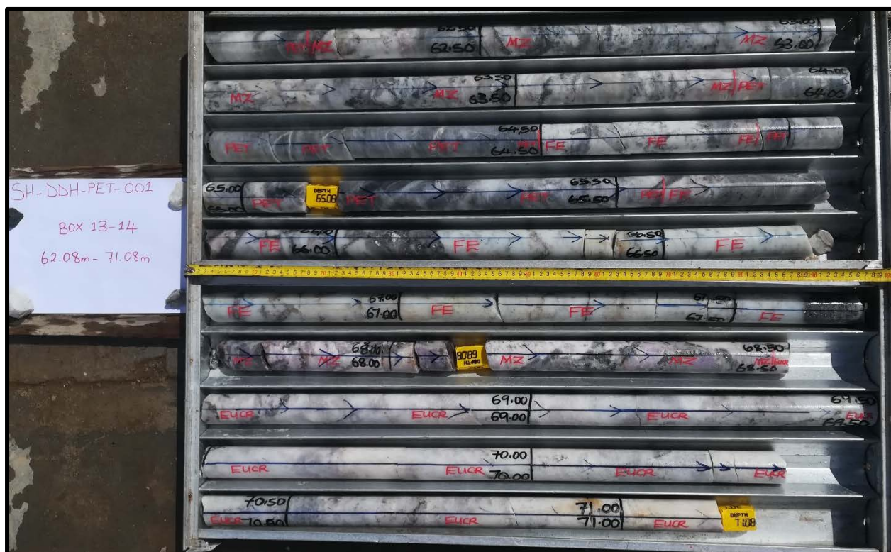
Figure 2.4: Preliminary diamond drill core photo from the Shaft pegmatite body showing how the different lithological boundaries were marked. Black lines show core orientation markings and black numbers represent the metre markings and red letters are abbreviations for the different lithologies.
