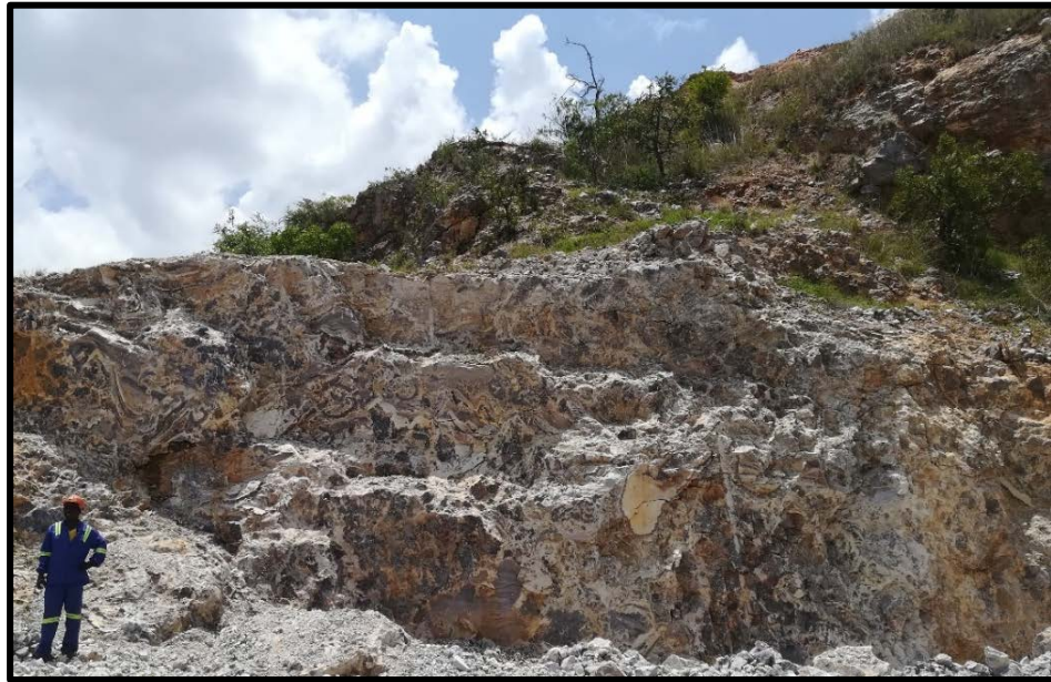
Figure 3.8: Typical Cobbled Zone which consists of a matrix of albite feldspar partly replaced by lepidolite forming spherical masses of various sizes within the Bikita quarry
