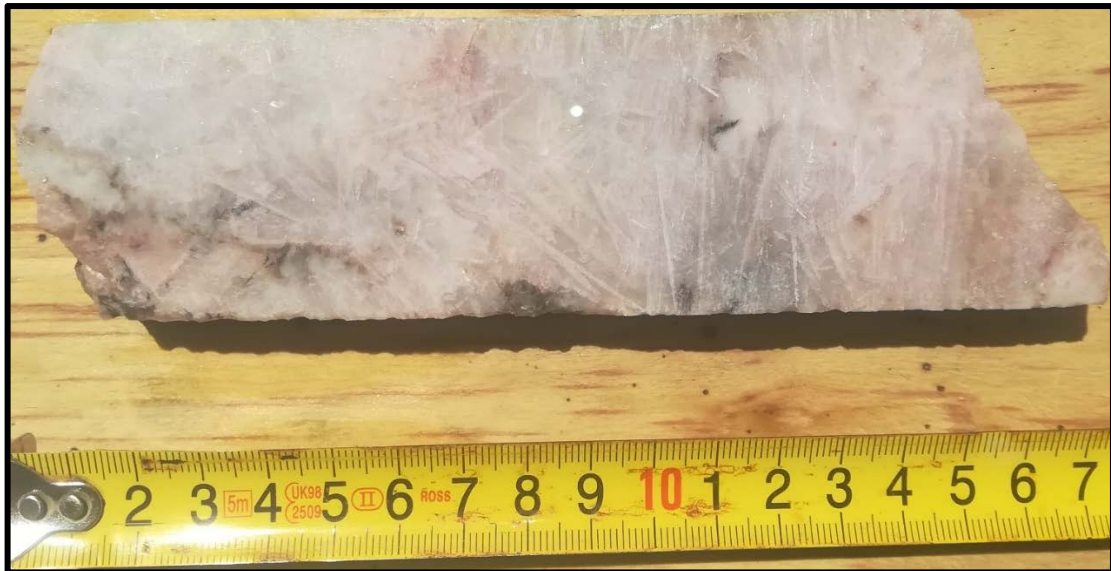
Figure 3.14: Core sample from the Spodumene pegmatite showing massive SQI indicated by the pink colour with distinctive elongated acicular crystals of spodumene
