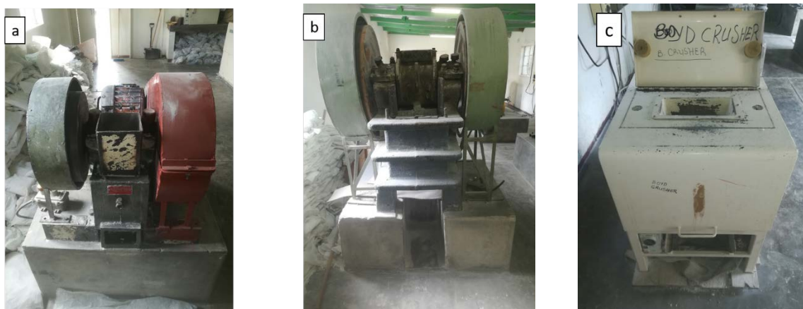
Figure 8.1: Laboratory crushing equipment. (a) Photograph of the -28mm jaw crusher (b) Photograph of the -150mm jaw crusher (c) Photograph of the Boyd Crusher
