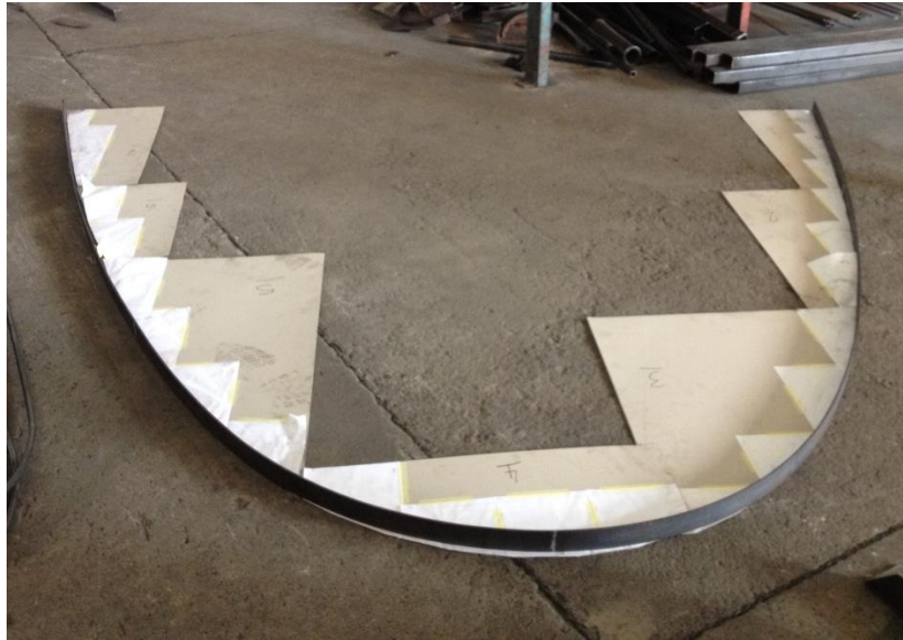
Figure 8-26: A stencil is used to determine the shape and guide the bending of the flat bars
