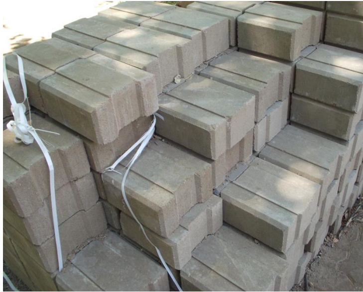
Figure 4-4: The Dry-stack Interlocking Blocks used in the construction of the prototype
