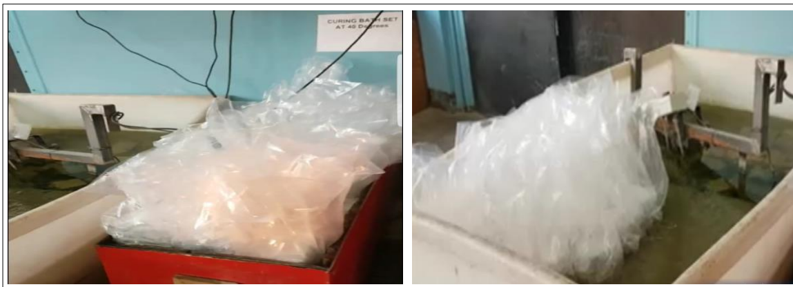
Figure 3.17: Plastic Wrapped Concrete Moulds in Curing Bath
