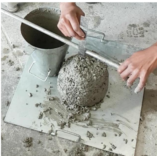
Figure 3.9: Slump for Concrete Mix 3 with Superplasticiser
