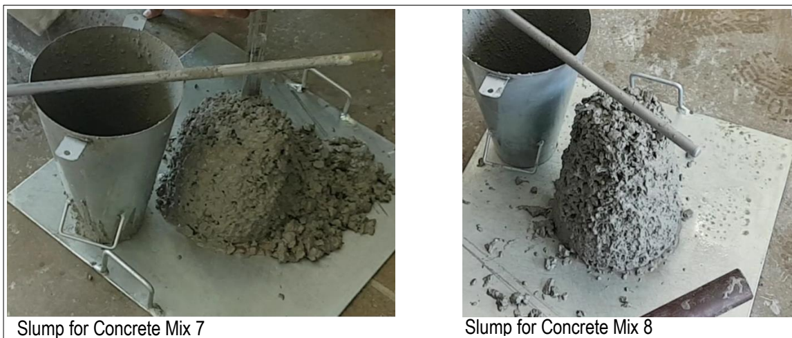
Figure 3.10: Concrete Slump for Mix 7 and 8 With Superplasticiser
