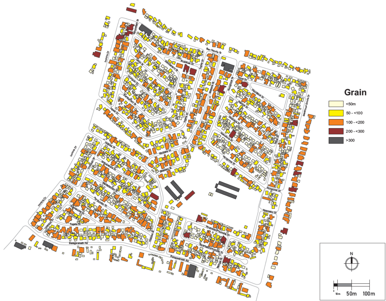
Figure 68: Grain and texture map. Grain refers to the size of buildings and texture refers to the extent to which different sizes are placed in close proximity
