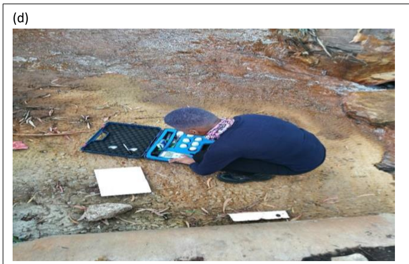
Figure 7: Images showing sample collection (a) Vaal dam sample collection, (b) sample collection at a spring, (c) purging of pipes linked to borehole before sample collection and, (d) taking physico-chemical parameters in situ.
