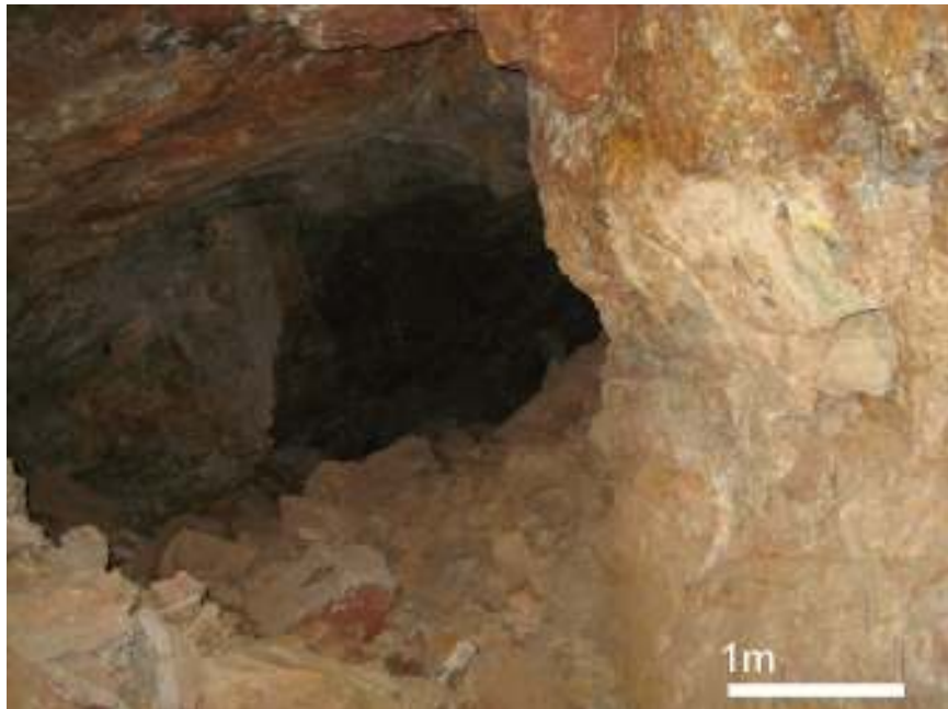
Figure C11: A typical example of the adits that were developed in the Witkoppies Gold Mine (Fig. C10, GR 307380- 7161742).
