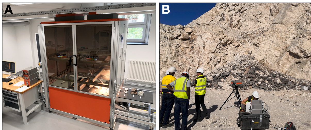
Fig. 3. Set-ups of the hyperspectral sensors in laboratory conditions as well as in the field. (A) The laboratory rock scanner set-up (or SisuRock configuration) with the AisaFENIX and AisaOWL mounted inside. Samples and/or drill-cores are placed on the moving stage in order to be scanned by both sensors. (B) The AisaFENIX mounted to a tripod for in-situ outcrop scanning at the V1V2 open pit. A workstation with a personal computer is required and powered by a mobile generator.
