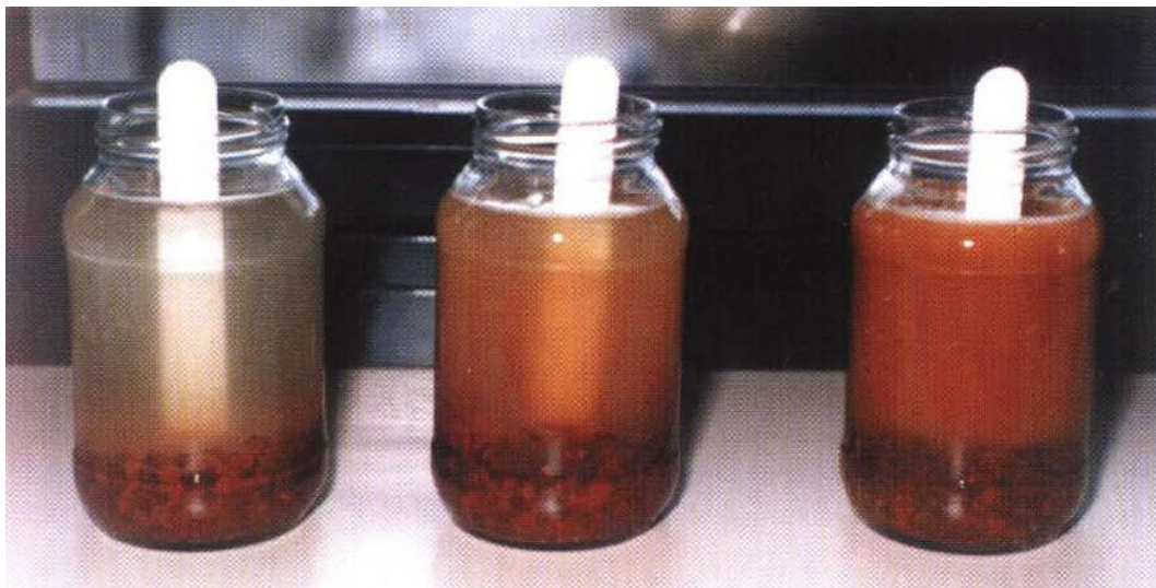
Figure 15: Estimating turbidity using spatula visibility showing non-sodic soil on the left, moderately sodic soil in the centre and strongly sodic soil on the right (Rengasamy and Bourne, 1997).
