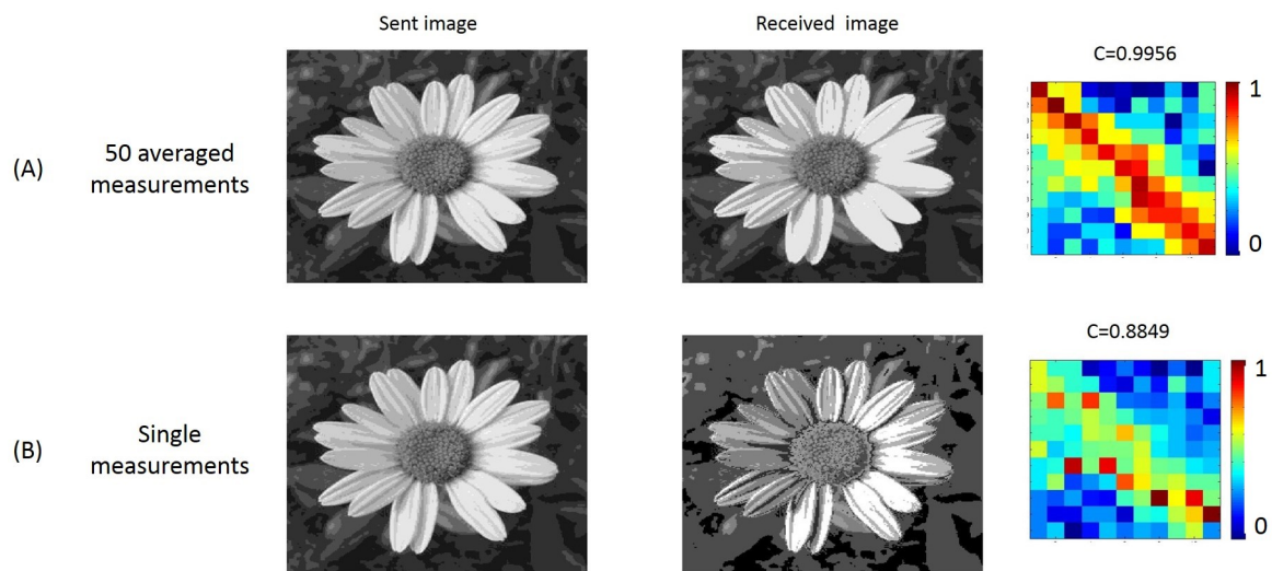
FIGURE 4.7: Simulation of data transfer using the crosstalk matrix that was over (A) 50 measurements and also (B) data transfer over a single measurement. The correlation between sent and received image was 0.9956 as compared to a single measurement with 0.8849.
