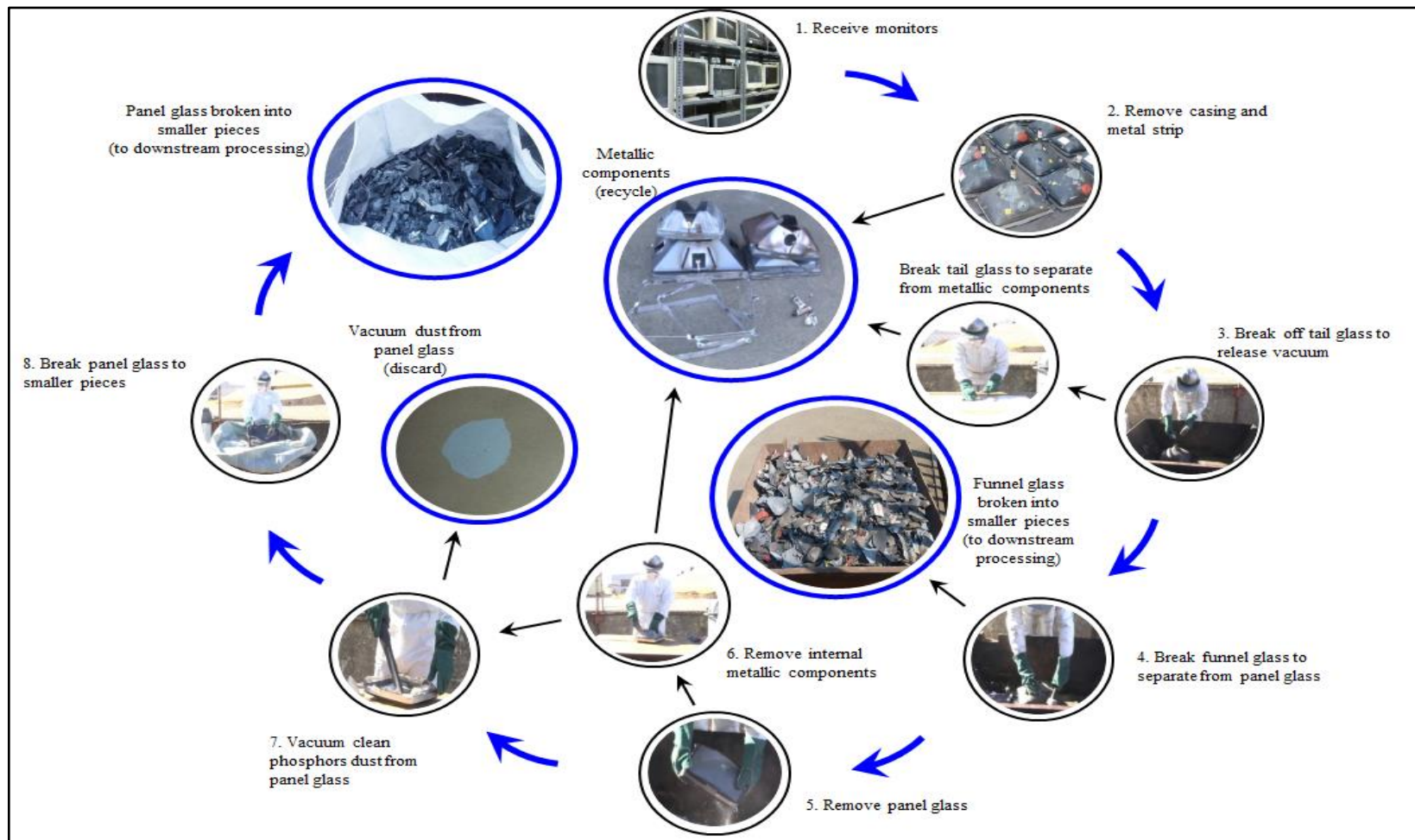
Figure 87: Process flowsheet illustrating the step-wise procedure for the manual separation of CRTs
