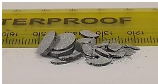
Figure 39: Fractured green compact fabricated from overaged 2124-Al with 10% \text{Al}_2\text{O}_3 powder.
