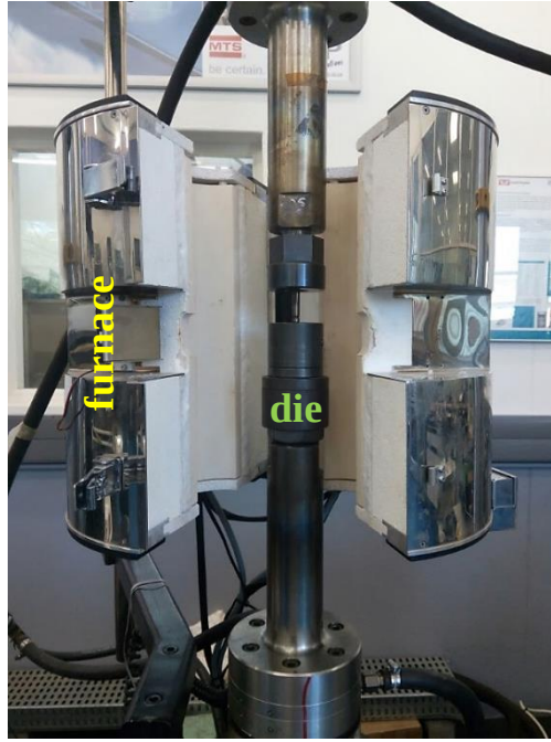
Figure 13: Furnace and die for extrusion experiments.
