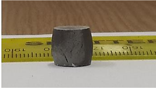
Figure 64: 2124-Al with 10% SiC sample which was sintered at 490°C for 1 hr, soaked at 280°C for 20 minutes and uniaxially compressed at 280°C and strain rate of 5 \text{ s}^{-1} up to a total strain of 0.3.
