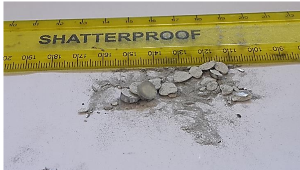
Figure 29: Fractured 2124-Al green compact after cold compaction.
