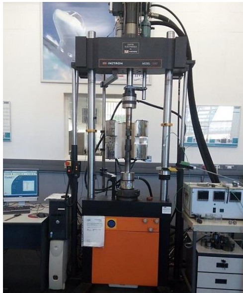
Figure 12: Die, Instron® press and furnace setup for extrusion experiments.
