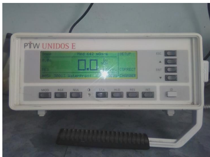
Figure 3.11 A PTW-Freiburg UNIDOS E universal electrometer used in this study to record charge readings.
