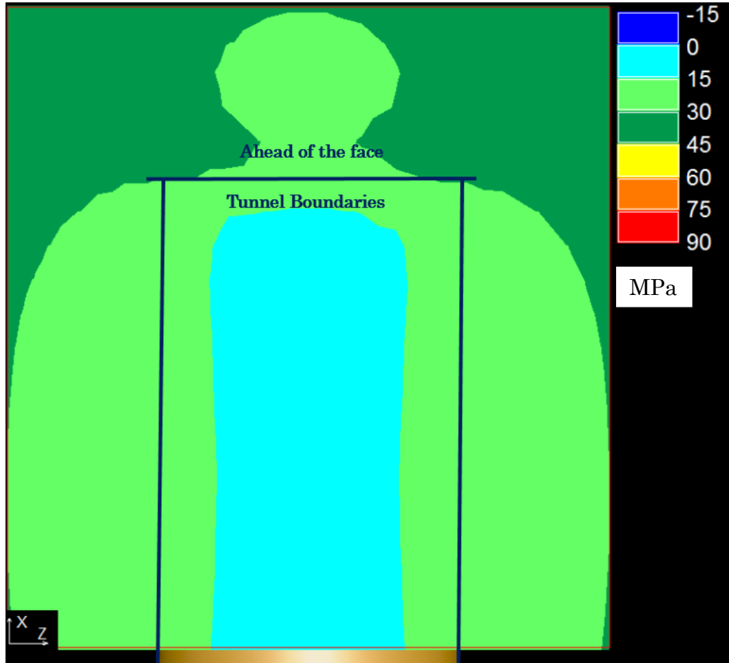
Figure 6.2.6: Top view of cutting plane depicting \sigma_3 distribution through the roof of an eight-metre diameter tunnel ( \sigma_x = 70 MPa, \sigma_y = 35 MPa, \sigma_z = 70 MPa).
