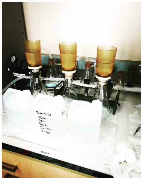
Figure 3.6: Filtration instrumental set-up used in sample preparation procedures.
