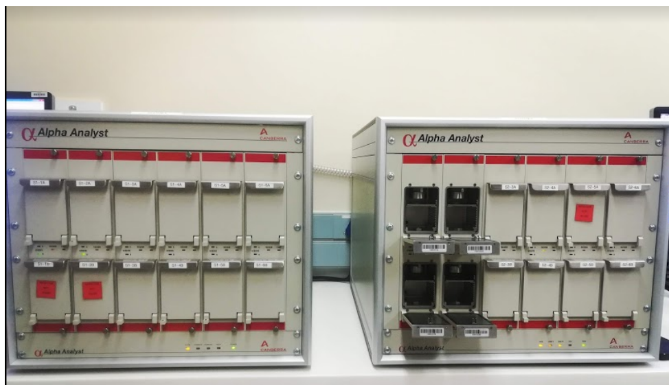
Figure 3.10: Alpha spectroscopy chambers manufactured by CANBERRA
