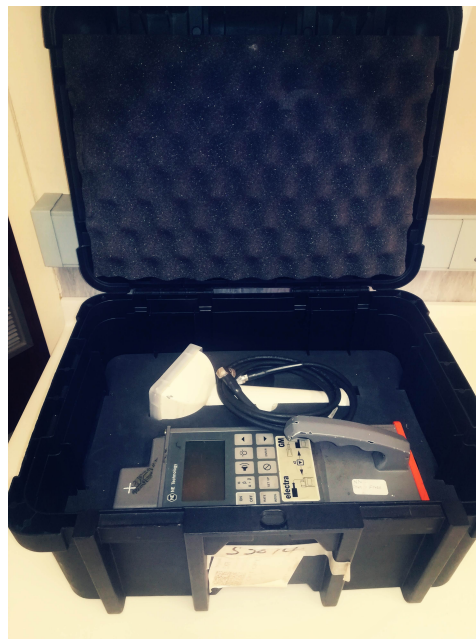
Figure 3.4: An Electra Gm used for background radiation level and surface radiation level on containers.
