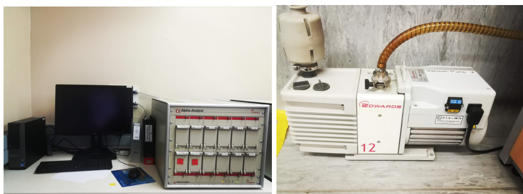
Figure 3.11: LHS: display with Genie 2000 software. RHS: Vacuum pump
