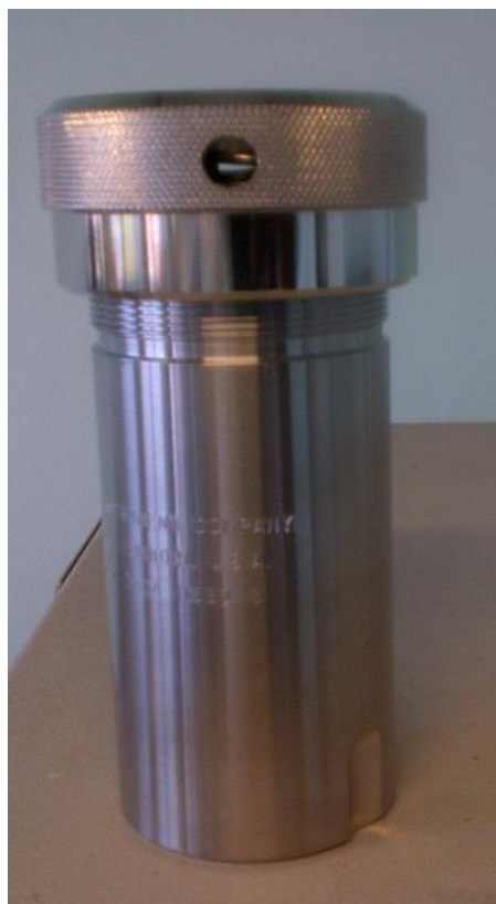
Figure 3.2: Autoclave used for zeolite NaY synthesis in this study
