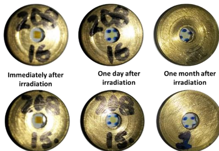
Figure 5-2: Fading of discolouration observed in ~25 MGy irradiated EJ208 samples.
