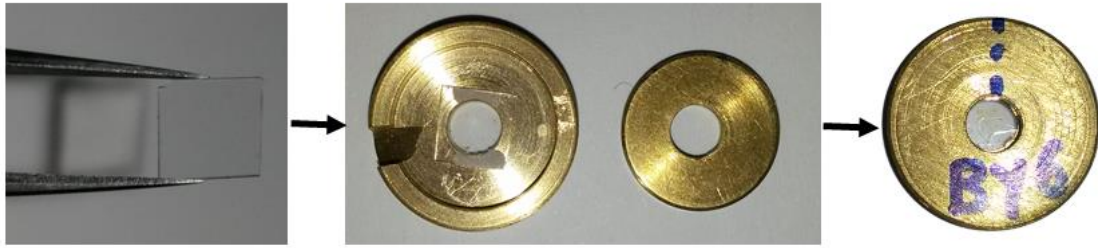
Figure 4-6: The final product of a polished sample, and a sample mounted into the brass holder.
