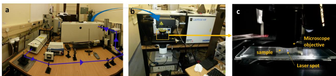
Figure 4-12: (a) Back view showing the path travelled by the laser into the LabRAM HR, (b) front view of the spectrograph, (c) zoomed view of the sample undergoing fluorescence.
