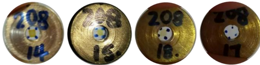
Figure 5-1: EJ208 samples irradiated to doses of ~80 MGy, 25 MGy, 8 MGy and 0.8 MGy from left to right.
