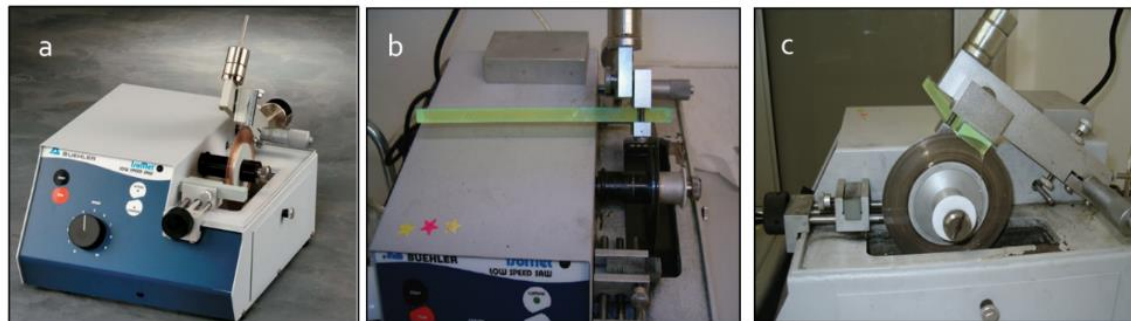
Figure 4-3: Photographs of (a) the Buehler IsoMet cutting machine, (b) a front view of an EJ260 bar being cut, (c) a side view of the EJ260 bar being cut.
