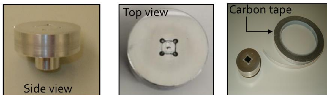
Figure 4-4: Aluminium holders used to mount the samples onto before polishing.
