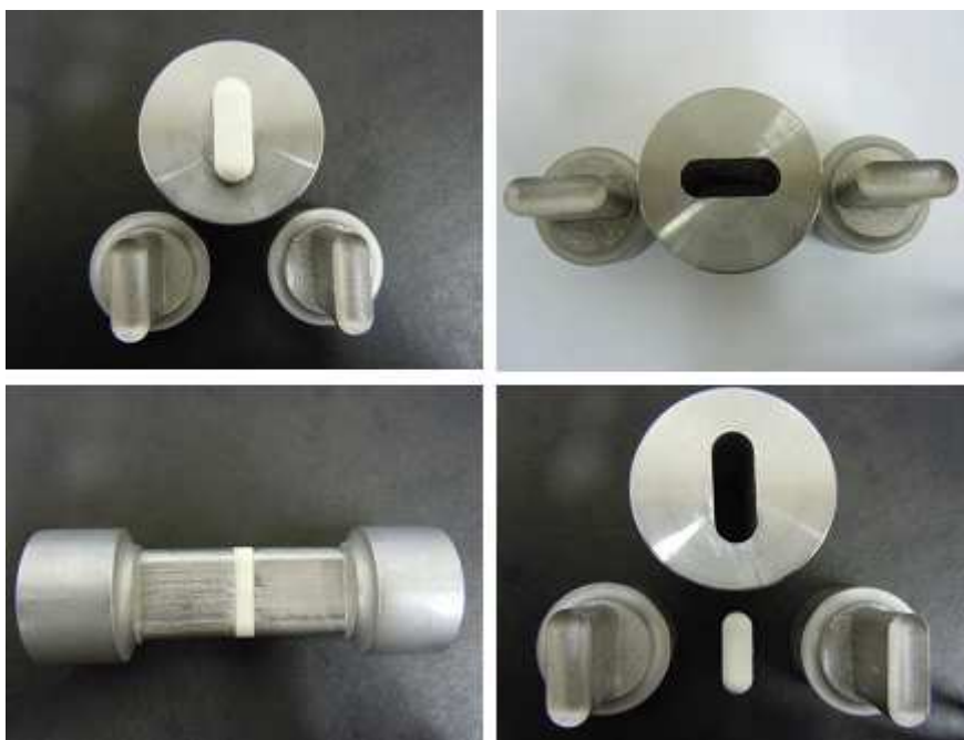
Figure 5.1: Digital photographs of the steel punch and die set and a polymeric caplet punched using the set.
