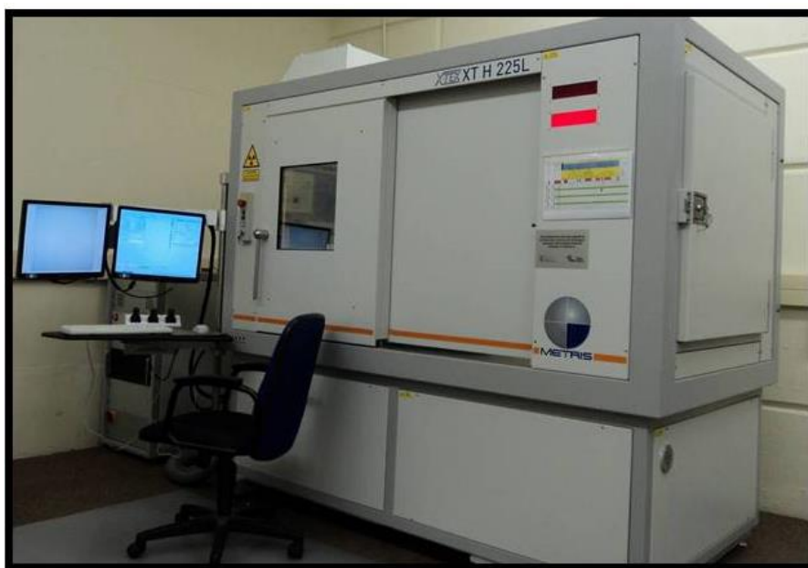
Figure 3-33 X-TEK XT H 225L tomographic imaging System at NECSA
