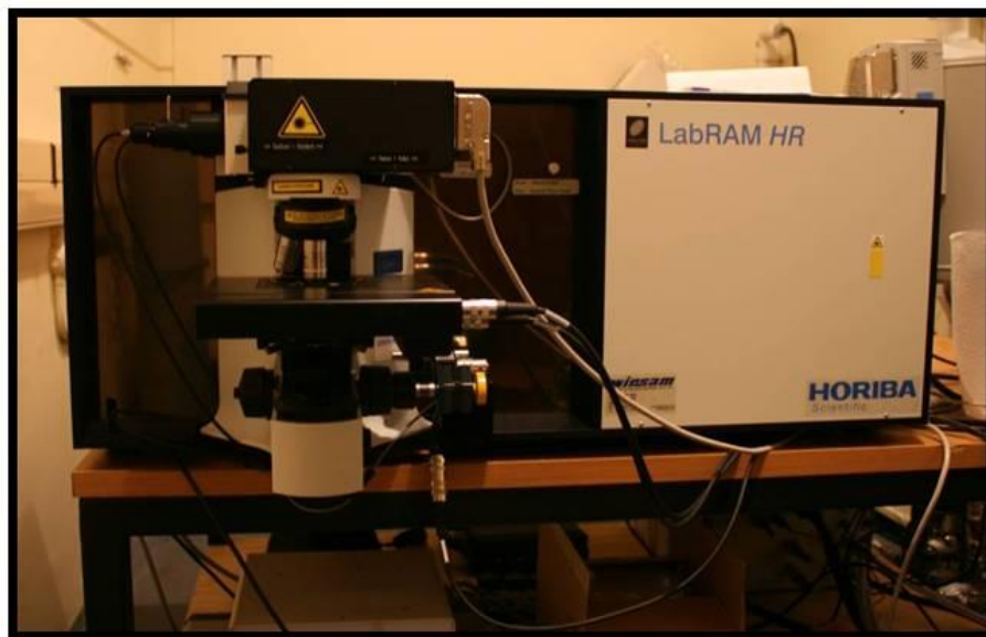
Figure 3-27 LabRAM HR instrument used for Raman Spectrographic tests
