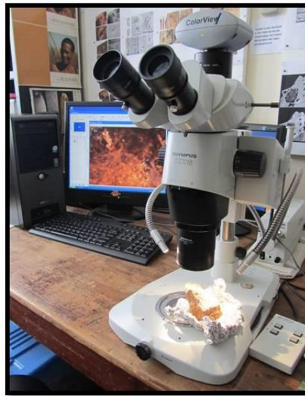
Figure 3-21 Multifocal Leica Z6 APO microscope, fitted with a digital camera, used to acquire light microscopic images (pictured here imaging the MH2 mandible specimen)
