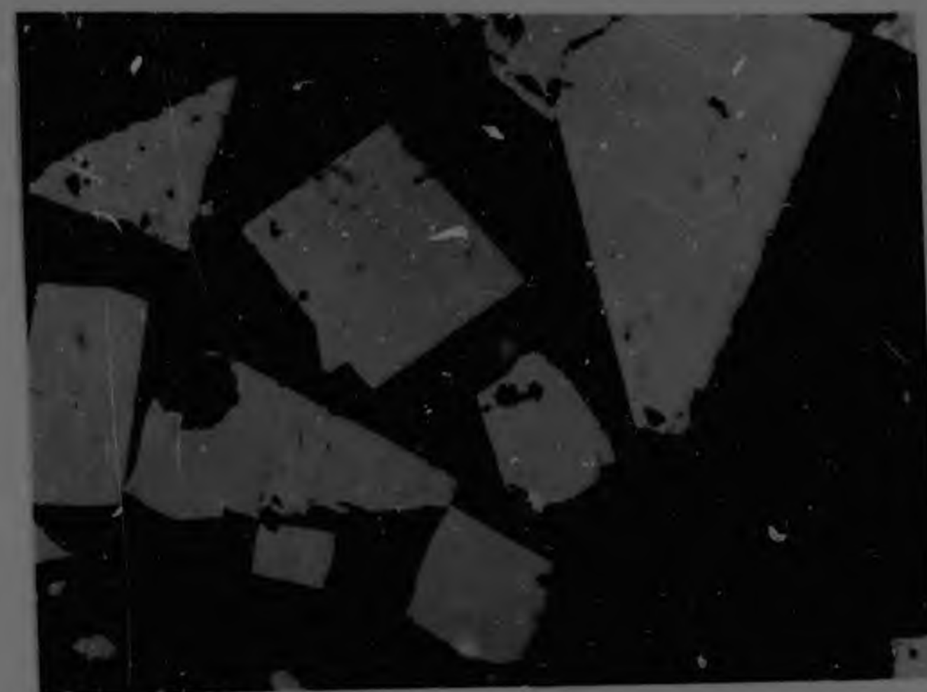
Fig. 28. Variety of crystal shapes shown by arsenopyrite.
