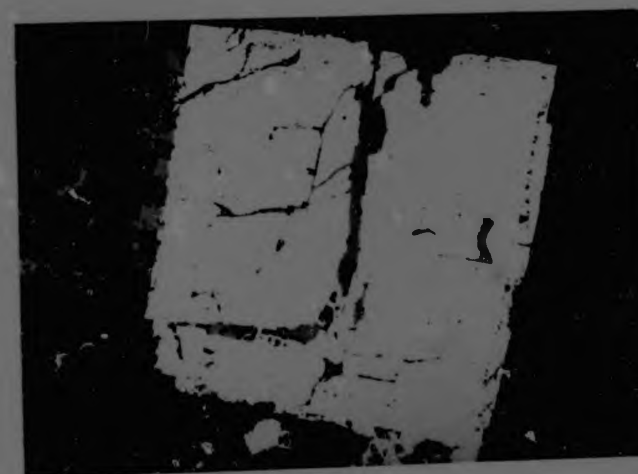
Fig. 37. Sphalerite (grey) filling fractures in a crystal, arsenopyrite and as irregular patches along the boundaries of the crystal. X 150
