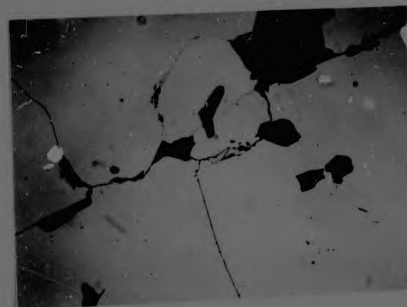
Fig. 33. Chalcopyrite (light grey) formed between interlocking grains of arsenopyrite.
