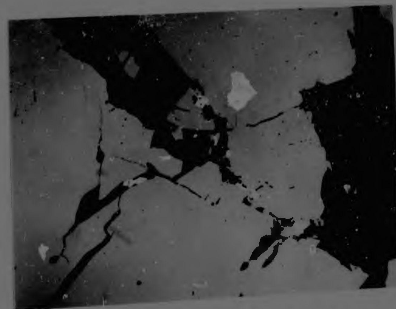
Fig. 35. Gold (white) between crystals of arseno- pyrite and as thin veins filling cracks in the arsenopyrite.
