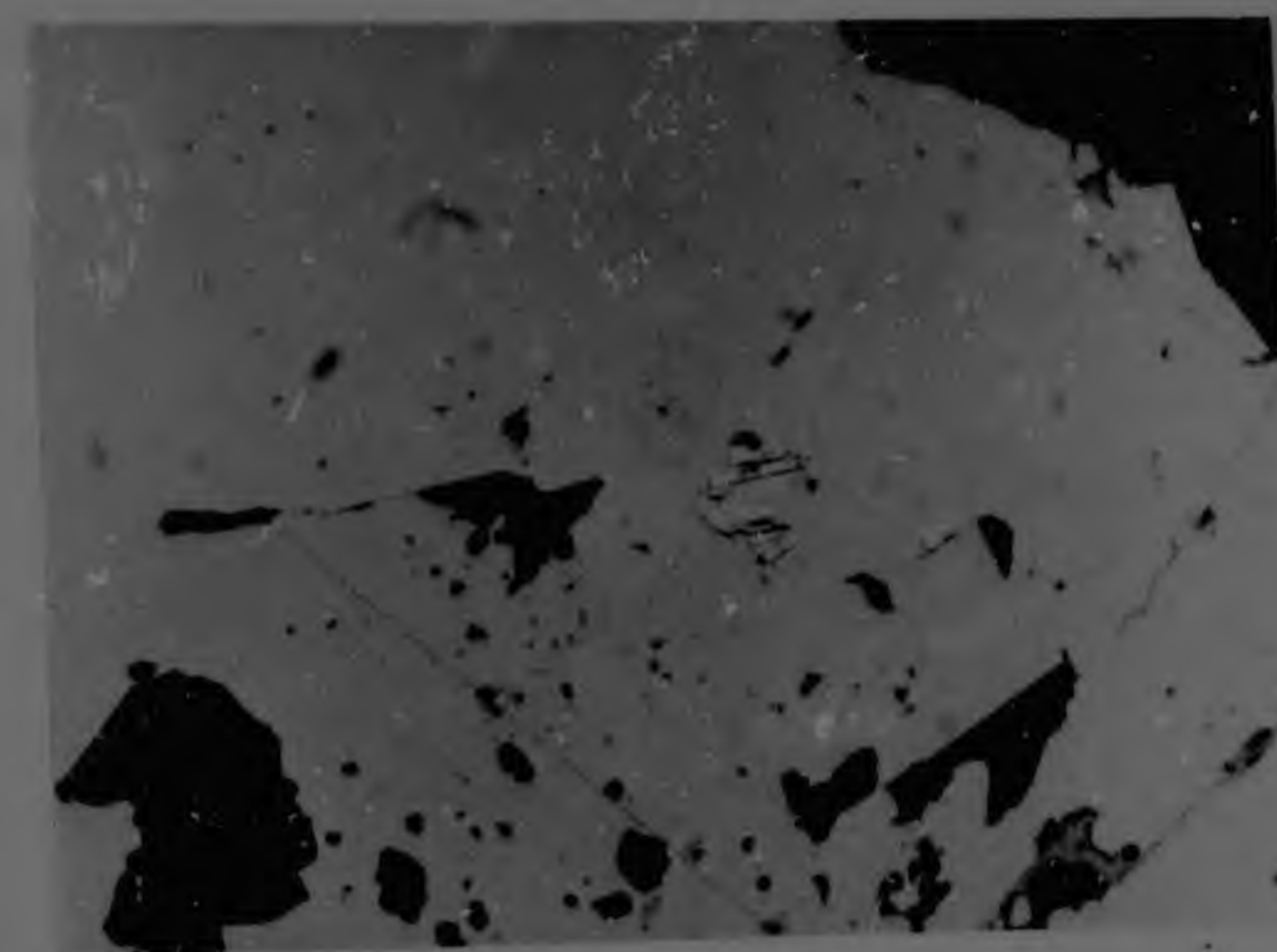
Fig. 34. Gold (scratched) enclosed in arsenopyrite. Chalcopyrite (light grey) filling fractures in the arsenopyrite.
