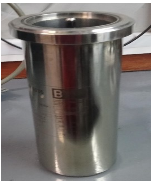
Figure 3-3C: Stainless steel reactor vessel. Key.
