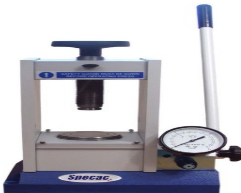
Figure 3-4: Manual Hydraulic Laboratory Pellet Press (Specac, 2018).
