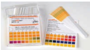
Figure 4.2 Universal indicator paper used to measure pH
