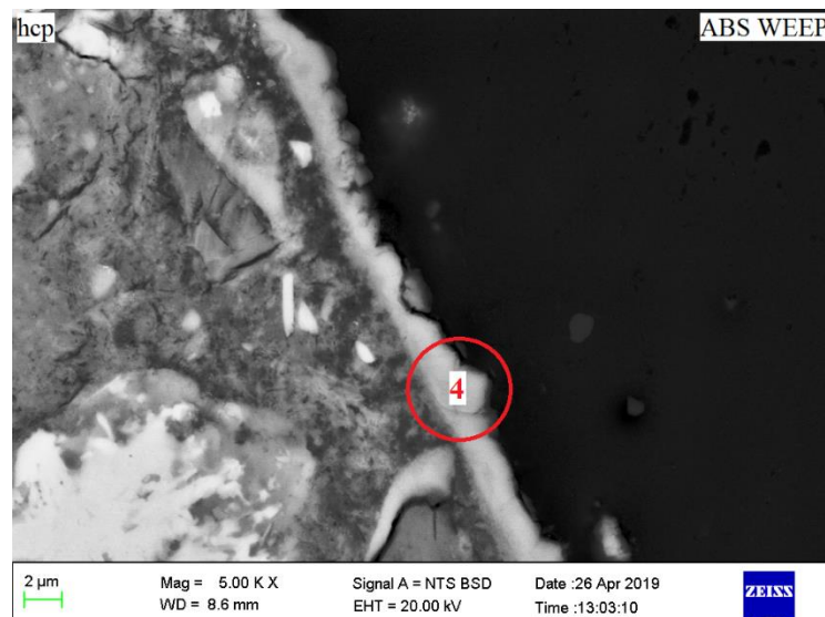
Figure 58: BSE of ABS WEEP in PCM(Blend-30) at 5 000 times magnification.
