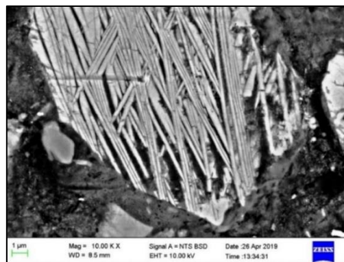
Figure 67: Crystal formation of belite and C-S-H at 10 000 times magnification.
