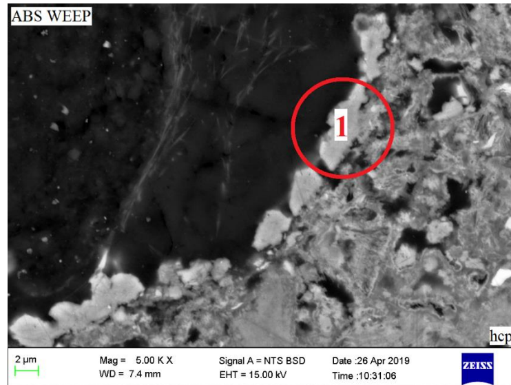
Figure 54: BSE image of ABS WEEP in PC(Blend-30) at 5 000 times magnification.
