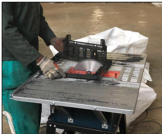
Figure 11: Desco worker sawing WEEP into smaller fractions. (Source: Desco, 2019).
