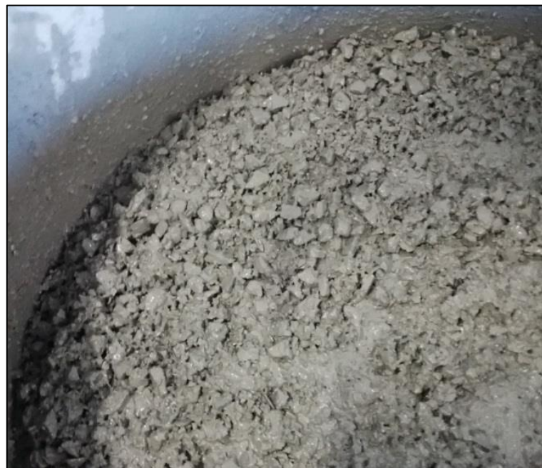
Figure 39: Segregation of aggregates of PCM(PC/ABS-30).
