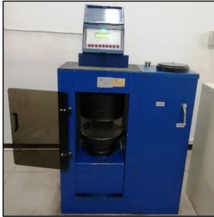
Figure 41: Cube press-foote machine (LHS) and a concrete cube between the steel platens (RHS).
