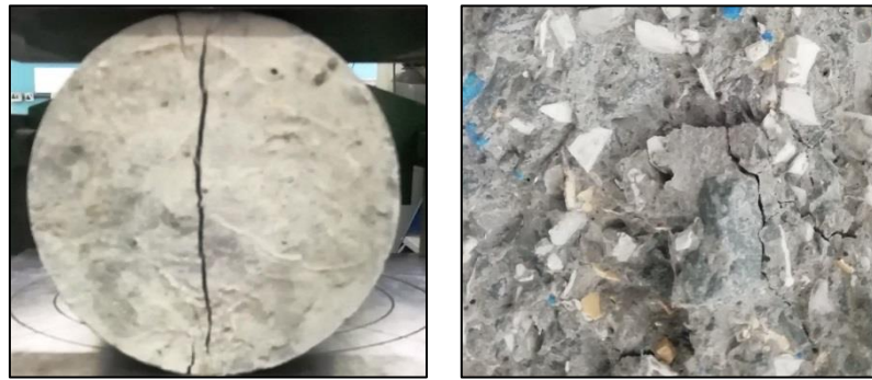
Figure 106: Tensile splitting of PC(Blend-30) (LHS) and the internal distribution of PC(Blend-30) (RHS).
