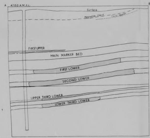
Transverse Section Showing Extent of Fibre Concentration
