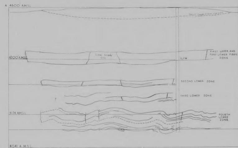
Transverse Section Showing Fibre Concentrations Coloured Red
