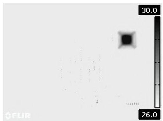
(d) Infrared image of ADC board with short circuited ADC.
