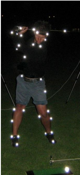
Figure 2.4: The position of the retro-reflective markers.
