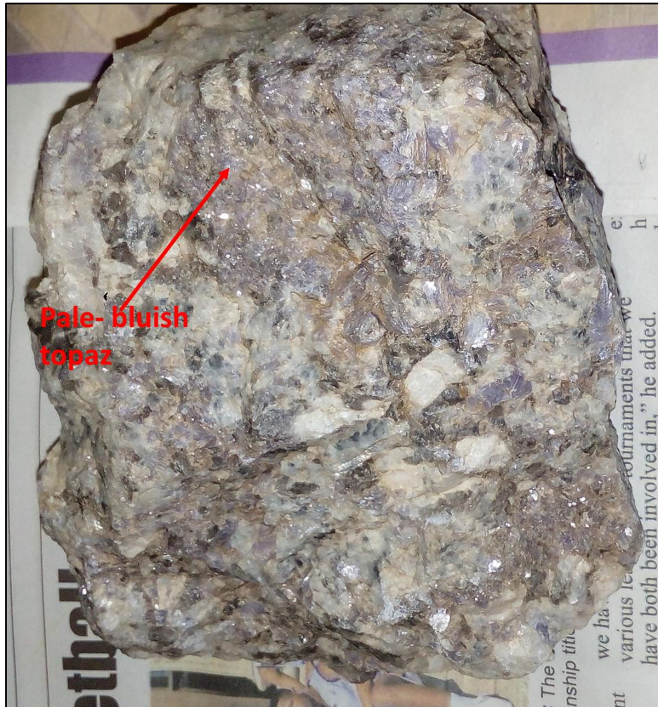
Figure 4. 5: Image of sample showing the topaz with bluish quartz from the western pit but it gives a true representation of how the topaz occurs in the Mbeta pits. Sample number MB03. (GPS Location: 35K 679529 E 7644 816N).
