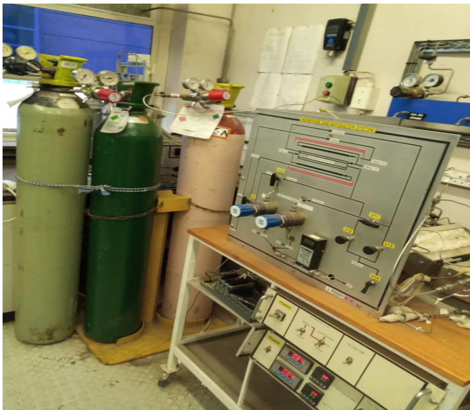
Figure A. 4 Picture of feeding cylinders to the membrane gas separation testing rig
