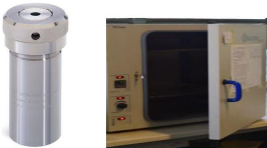
Figure A. 1 A 45 mL capacity autoclave (left) and LABOTEC EcoTherm® oven (right)
