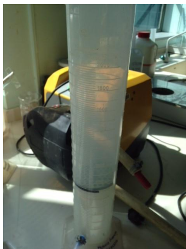
Figure 3.2 Laboratory scale leach bed reactor (LBR)
