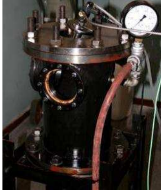
Figure 4.1: Constant volume pressure chamber
