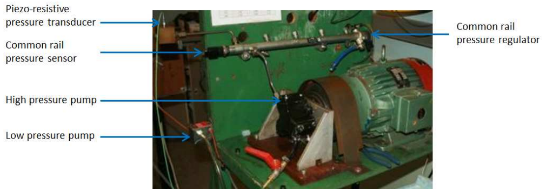
Figure 4.3: Common-Rail system driven by AC motor
