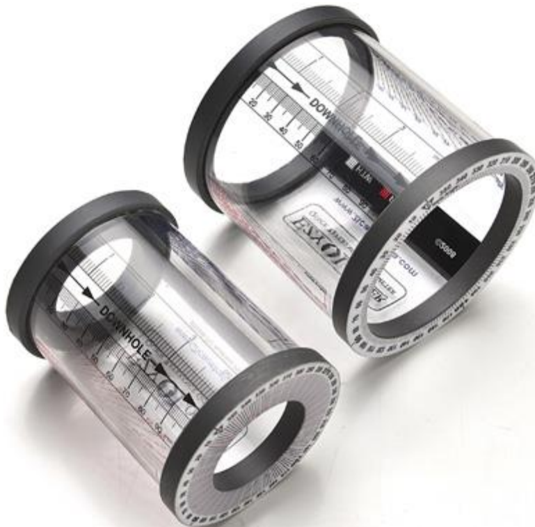
Figure 3-11 A goniometer for measuring alpha and beta angles (Westernex, 2018)
