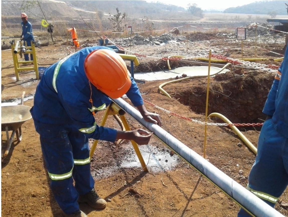
Figure 3-9 Drawing the orientation line along the entire length of the drill core extending it from the bottom of core mark (Courtesy of Pickstone-Peerless Mine).
