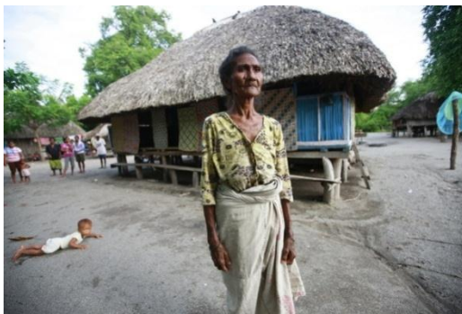
Figure 5.5 showing a wooden house on wooden columns to prevent damp floors, and to overcome mild floods in Suai Loro in Timor-Leste. Source: Copyright: UN-HABITAT/ Perret (2011)
