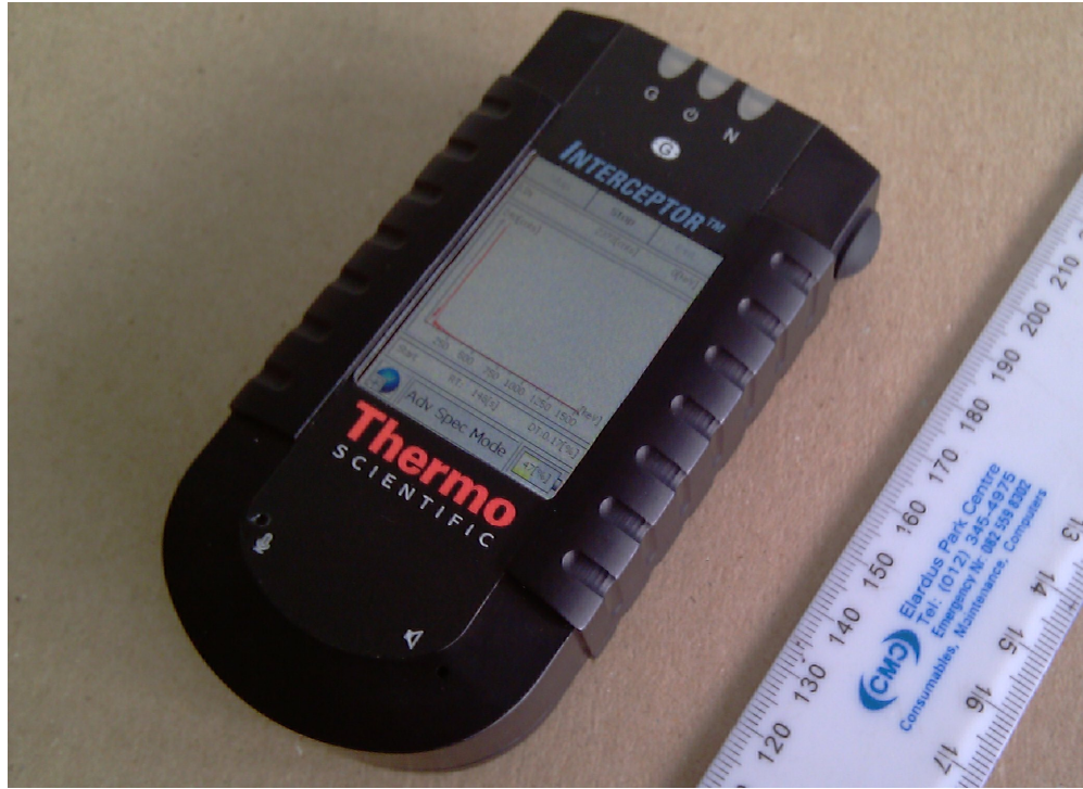
Figure 3.2 : Thermo Electron Corporation's Interceptor portable radiation detector.
