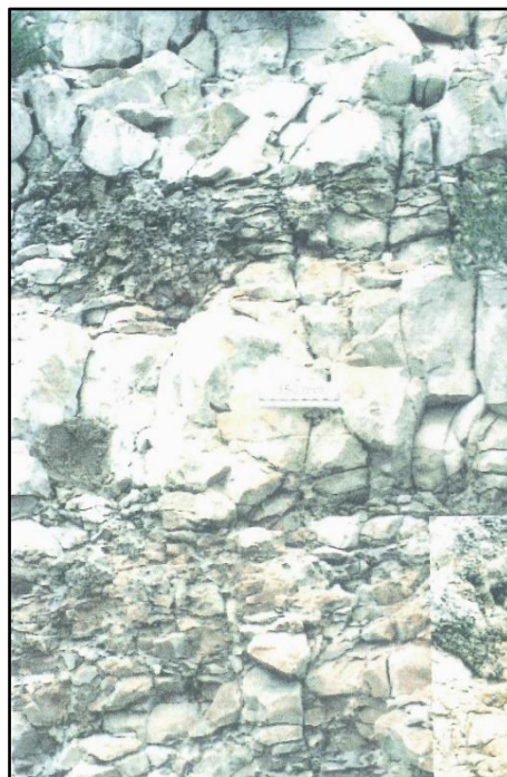
Figure 5.8: Jointing of the sandstones of the Eden Formation, with calcretisation of some of the weathered sandstone having taken place (after Haddon, 2005)
