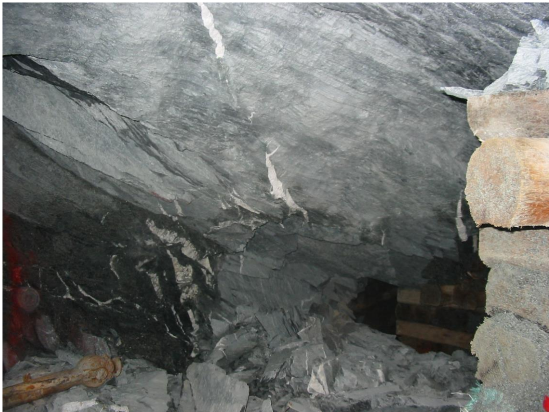
Figure 2-12 Photograph in stope showing WAF laminations
