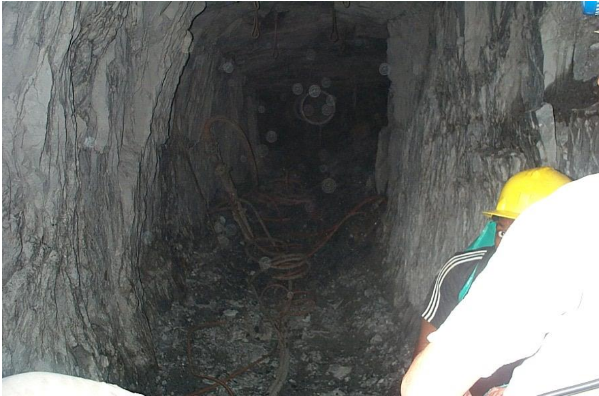
Figure 6-15 Photograph showing a development raise with WAF hangingwall before the production blast
