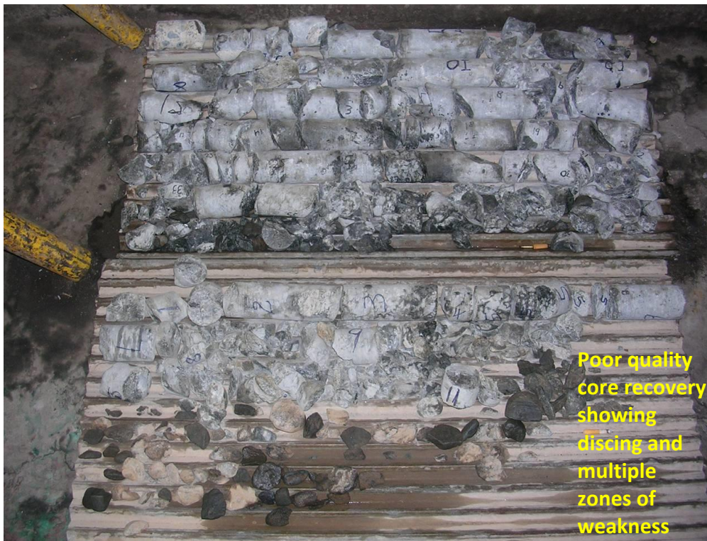
Figure 4-5 Drill core from WAF hangingwall geotechnical hole at Ya Rona shaft
