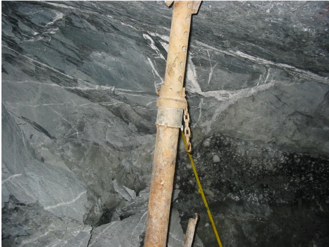
Figure 2-11 Photograph showing multiple planes of weakness and shearing of the WAF rockmass
