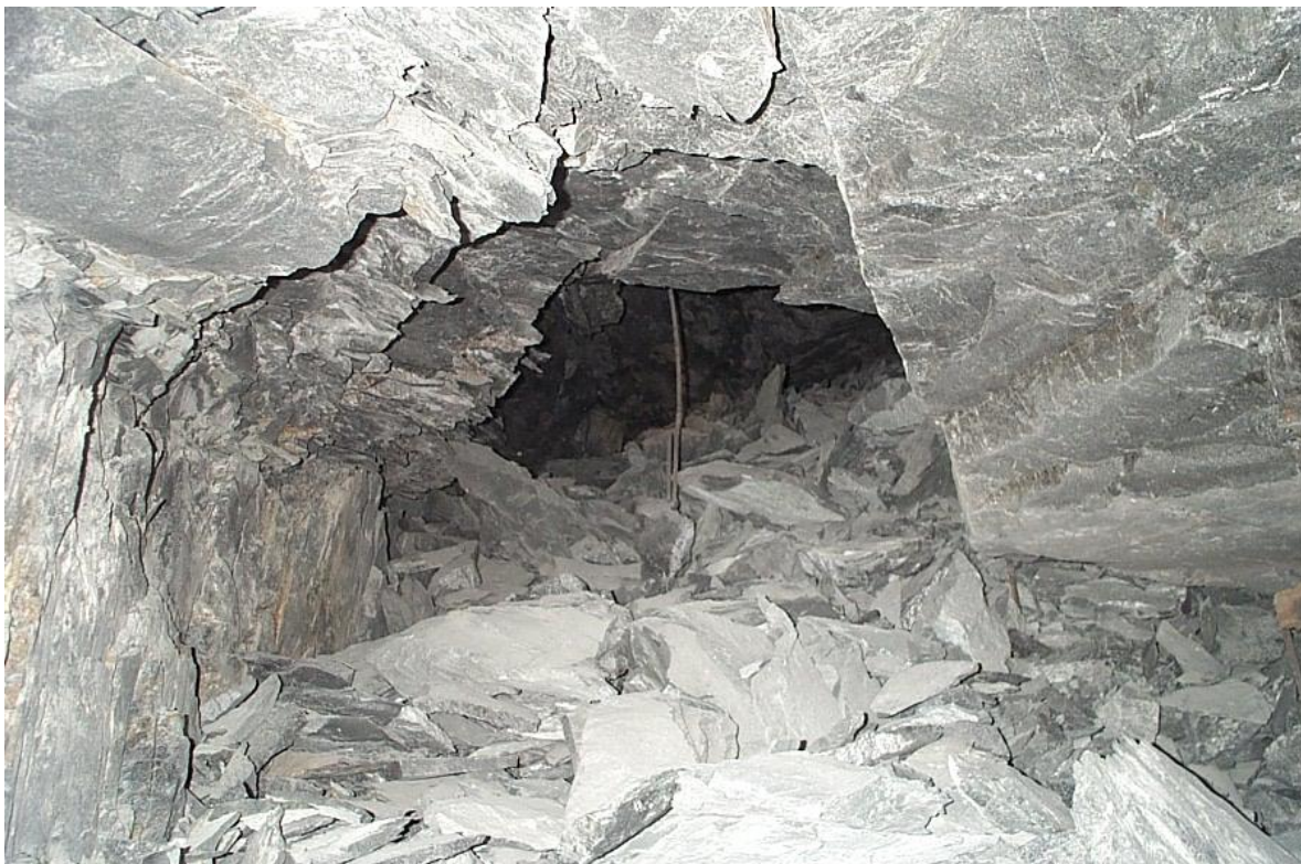
Figure 6-16 Photograph showing the same development raise in figure 6-15 after the production blast
