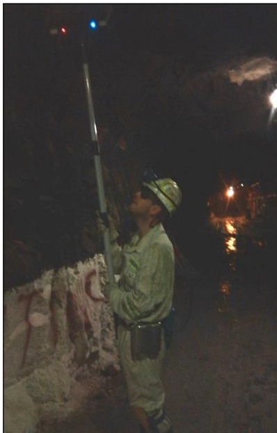
Figure 4.9: The author conducting GPR scans along the Roadway.
