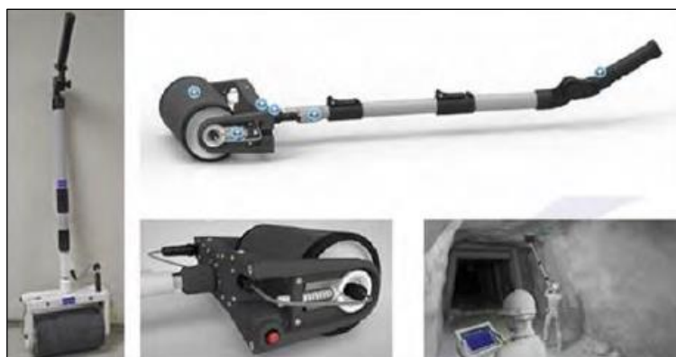
Figure 3.7: Sub Surface Profiler used for GPR analysis (Andrews, et al., 2019).
