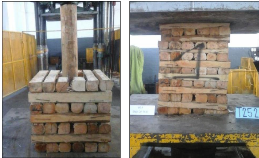
Figure 4.17: C-pack construction and testing at the CSIR Laboratory in Johannesburg.
