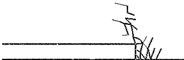
Figure 5.14 Perfectly plastic with high tensile strength; cohesion before failure = 20MPa; cohesion after failure = 20MPa; tensile strength = 20MPa
