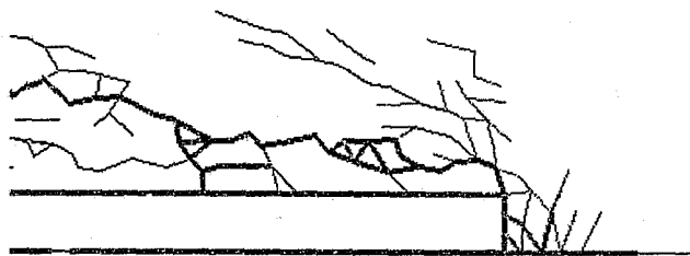
Figure 5.15 Perfectly plastic with low tensile strength; cohesion before failure = 20MPa; cohesion after failure = 20MPa; tensile strength = 1MPa
