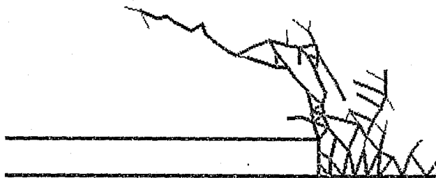
Figure 5.12 Cohesion softening with high tensile strength; cohesion before failure = 20MPa; cohesion after failure = 0MPa; tensile strength = 20MPa
