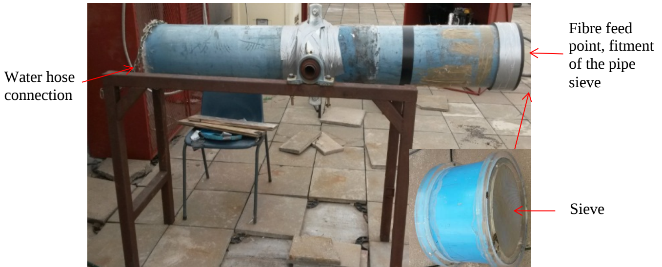
Figure 3.10 : Pipe mat rig in horizontal position
