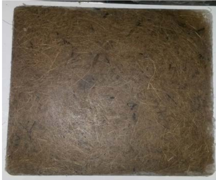
Figure 3.20 : An example of a fabricated composite specimen fabricated
