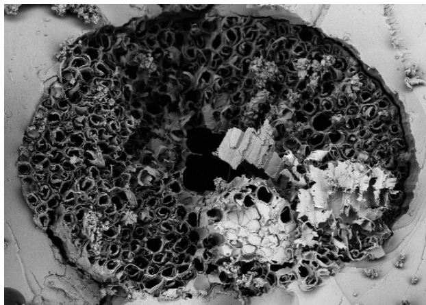
Figure 3.2 : SEM image of the coir fibre structure
