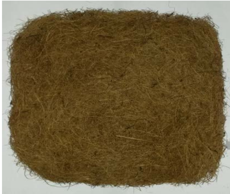
Figure 3.12 : Fabricated mat to be used for composite specimens
