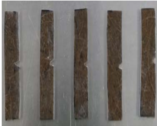
(b) : Impact testing specimens fabricated and prepared for testing
