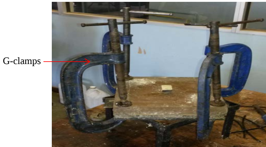
Figure 3.19 : G-clamps used to hold the male mould section in place
