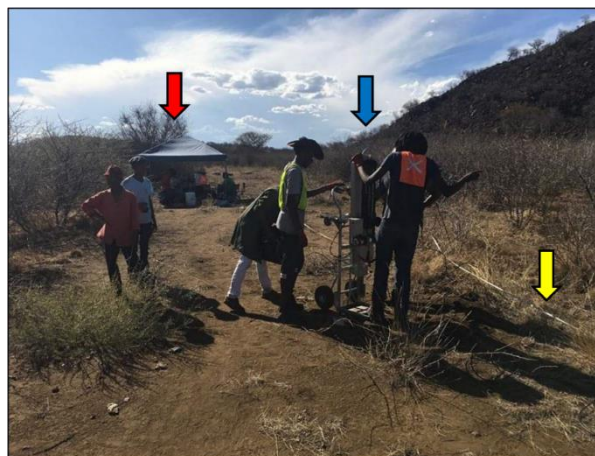
Figure 4.8: Survey layout along seismic profile 1 showing the weight drop (blue arrow), seismic station at the centre of the profile (red arrow), and the seismic profile with geophones (yellow arrow).
