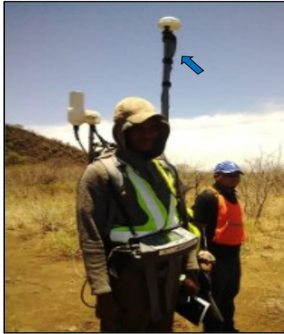
Figure 4.11: Caesium vapour walk magnetometer used for the magnetics data acquisition.
