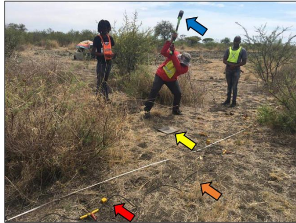
Figure 4.9: Geophones (red arrow), sledgehammer source (blue arrow), metal plate (yellow arrow), and the take-out cable (orange arrow) utilised during seismic data acquisition.
