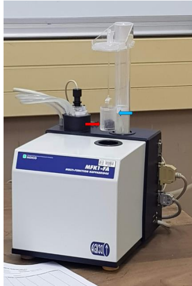
Figure 4.1: AGICO MFK1-FA used to measure the bulk magnetic susceptibility of the samples. Sample (red arrow) within the holder (blue arrow).
