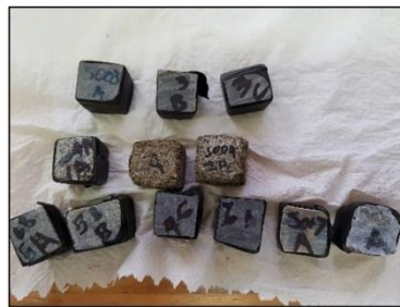
Figure 4.5: Rock samples wrapped with non-conductive tape to retain the moisture.
