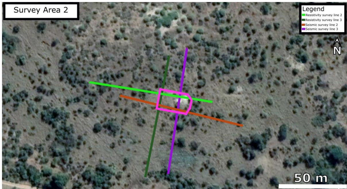
Figure 4.7: Area 2 with the resistivity profiles (orange and dark green lines, resistivity lines 2 and 3 respectively) and the seismic lines (light green and purple lines, seismic lines 2 and 3 respectively). Pink block in the figure indicates where the rock samples were collected (Google Earth Image).
