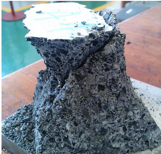
Figure 70. A coal-crete specimen of 100 mm square width and w/h = 1 after failure. The fractured sidewalls have been removed to expose the hourglass shape and the shear failure through the centre of the specimen.
