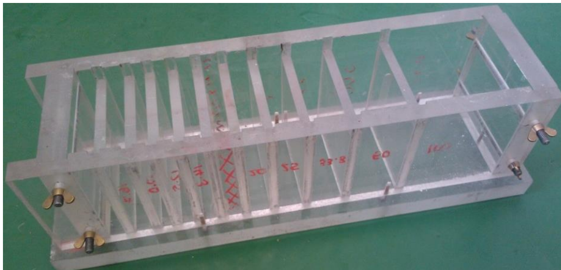
Figure 51. Mould for casting of 100 mm square specimens.
