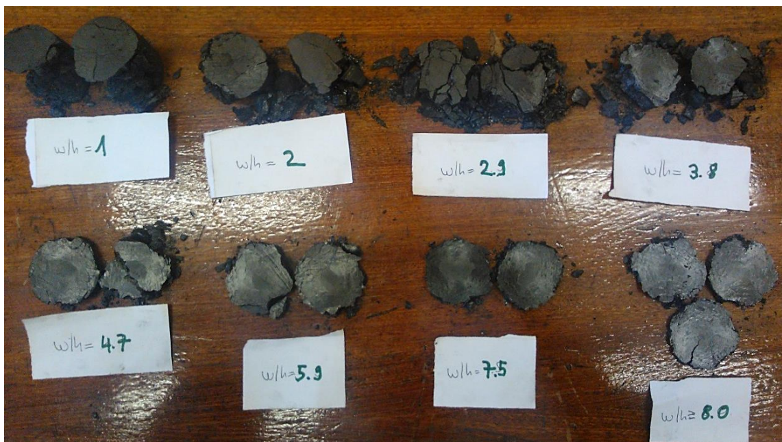
Figure 78. Coal specimens with various w/h -ratios after failure.
