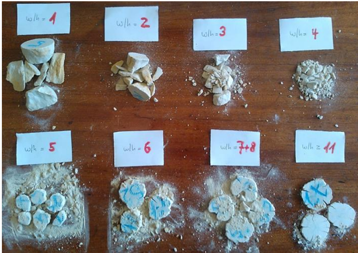
Figure 77. Sandstone specimens with various w/h -ratios after failure.
