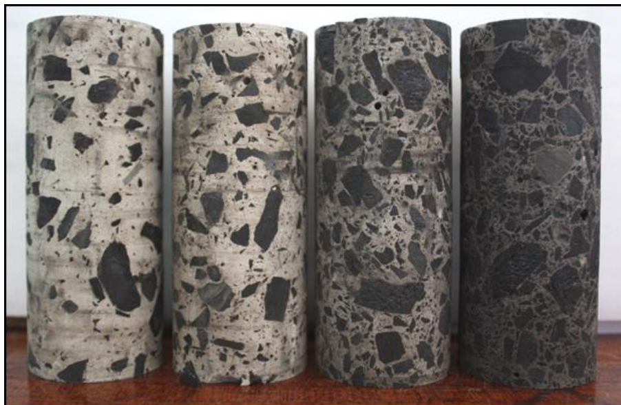
Figure 41. Specimens for UCS tests with 15%, 30%, 50% and 67% coal content (L-R).
