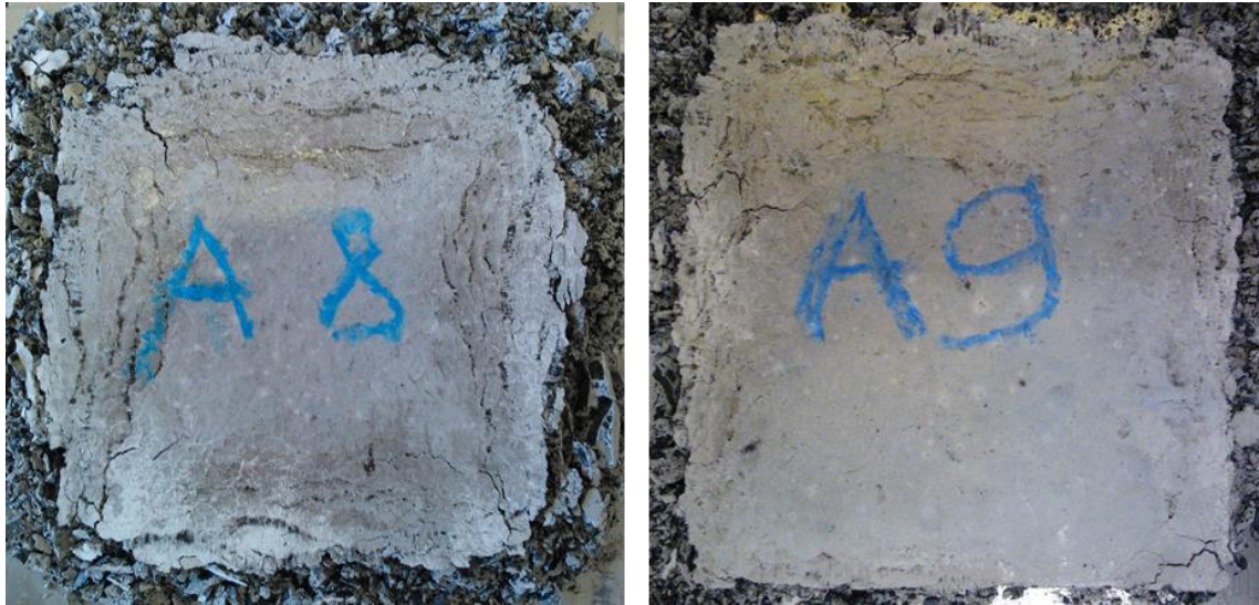
Figure 74. Coal-crete specimens of w/h = 7 (left) and w/h = 10 after compression.
