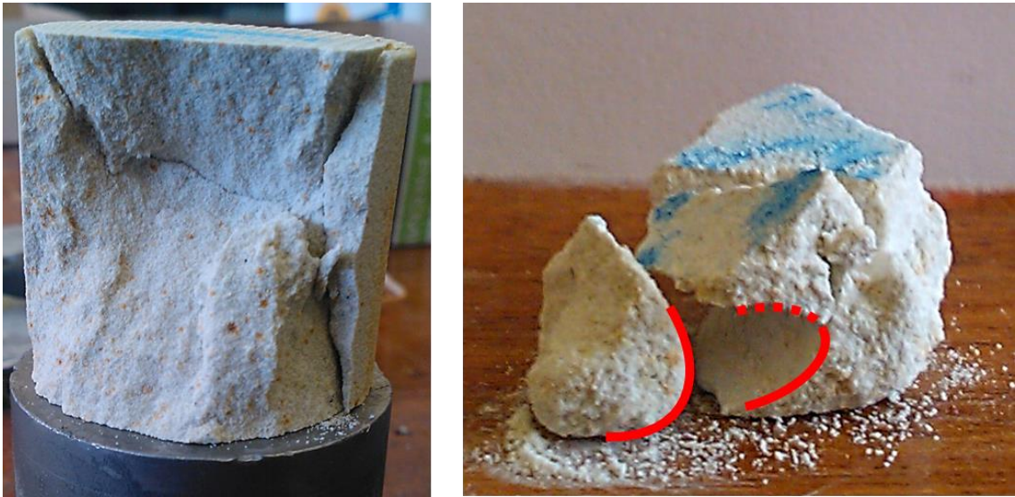
Figure 75. Double-cone type shear failure on a sandstone specimen of w/h=1 and wedging observed on a sandstone specimen core of w/h=4 .
