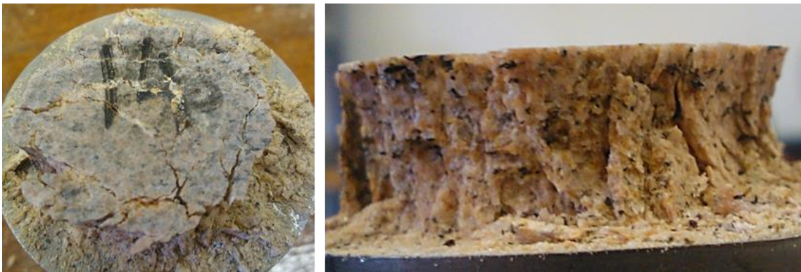
Figure 76. A granite specimen of w/h=3 after failure in top view (left) and side view (right).
