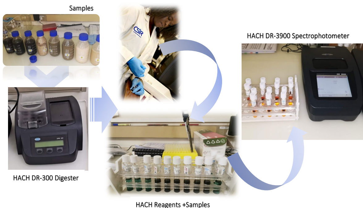
Figure 3.1: Spectrophotometric analysis method using standard Hach test kits
